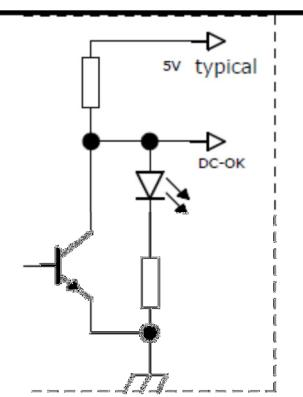
During normal operation, this signal is logic HIGH for output more than 85% (typical) of normal. Signal will go LOW for output less than 80% (typical) of normal. Green LED will light on PCB top side during normal operation.
