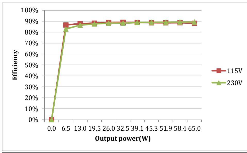
High efficiency is achieved by using QR technology. Synchronous MOSFETs or ultra-fast diodes are used as rectifiers in MB65S family.
