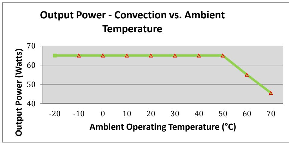
65W convection cooled at -20°C to 50°C operating ambient temperature. De-rated output power to 45.5W at 70°C.
