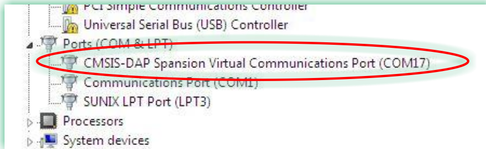
Figure 5: WyzBee™ CMSIS-DAP Debug Port Detection
