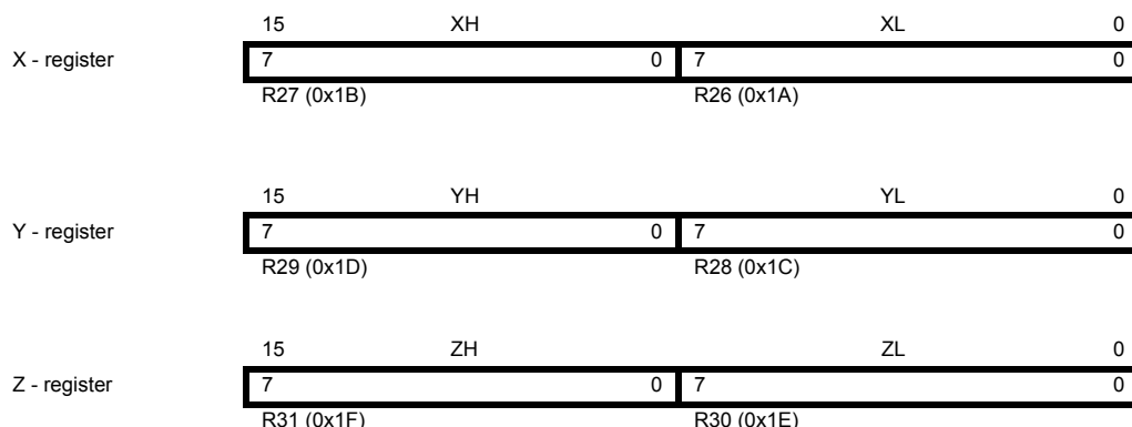
Figure 5. The X-, Y-, and Z-Registers
