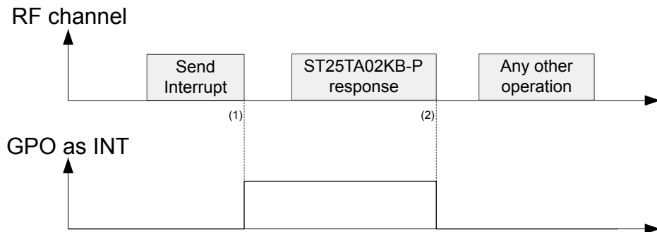
Figure 16. CMOS GPO configured as INT (GPO field = 0x40 or 0xC0)
