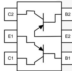
Figure 4. FMB2907A Internal Connections
