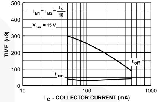
**Figure 14. Turn-On and Turn-Off Times vs. Collector Current**
