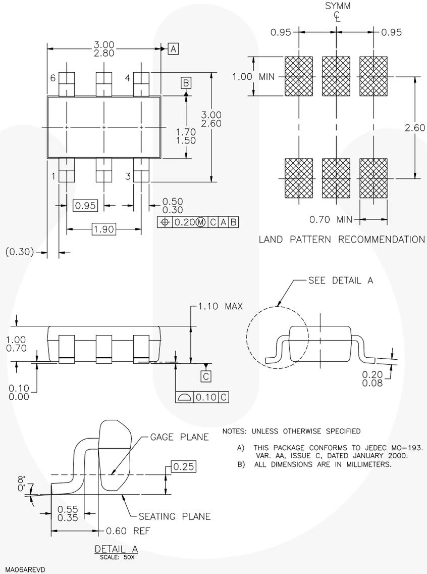
Figure 21. 6-LEAD, SUPERSOT-6, JEDEC MO-193, 1.6 MM WIDE (ACTIVE)
