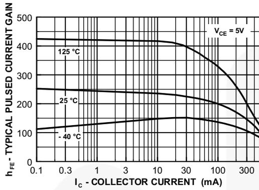
Figure 7. Typical Pulsed Current Gain vs. Collector Current
