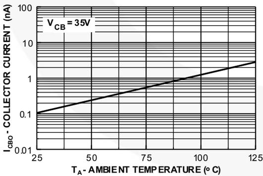
Figure 11. Collector Cut-Off Current vs. Ambient Temperature
