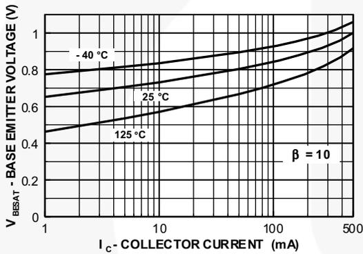
Figure 9. Base-Emitter Saturation Voltage vs. Collector Current
