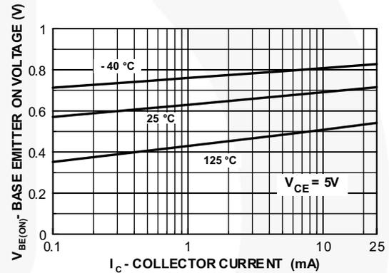
Figure 10. Base-Emitter On Voltage vs. Collector Current
