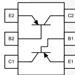
Figure 2. FFB2907A Internal Connections
