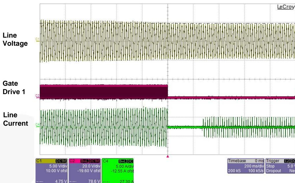
**Figure 29. Startup Slowly Increasing the Line Voltage**
