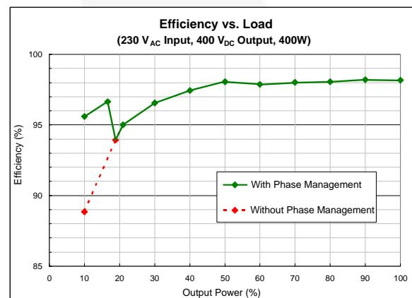
Figure 38. Measured Efficiency at 230 V<sub>AC</sub> (Default Thresholds)
