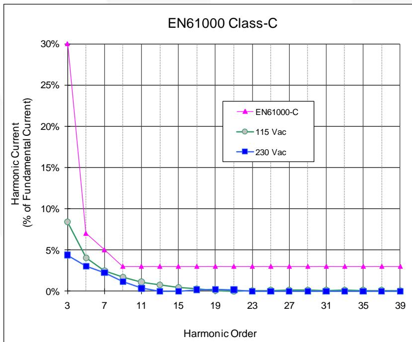
Figure 42. Measured Harmonic Current and EN61000 Class-C Regulation
