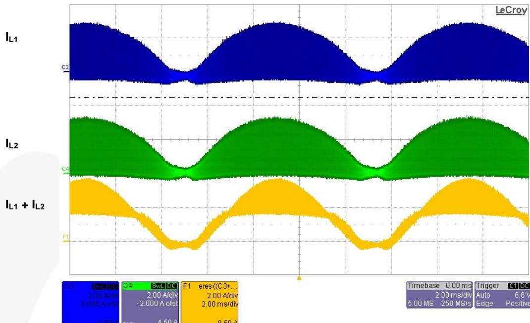
**Figure 21. Inductor Current Waveforms at Full-Load and 230 V<sub>AC</sub>**
