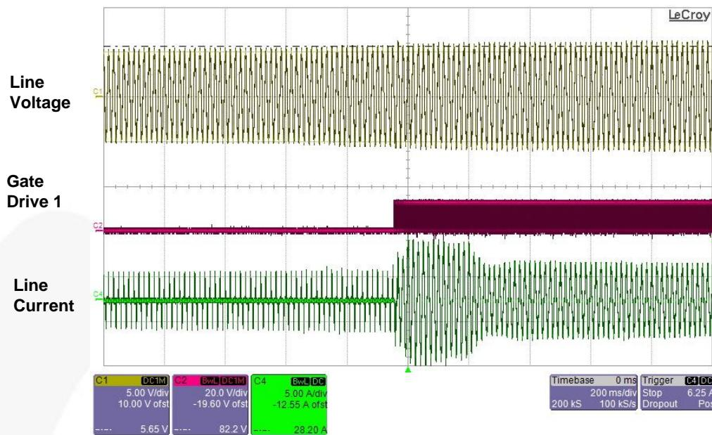
**Figure 27. Startup Slowly Increasing the Line Voltage**
