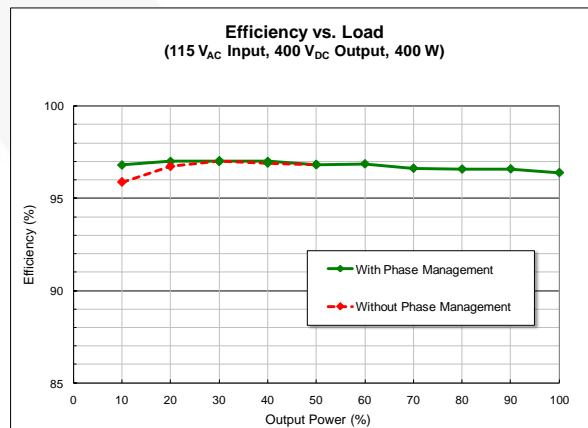
Figure 39. Measured Efficiency at 115 V<sub>AC</sub> (Adjusted Thresholds)
