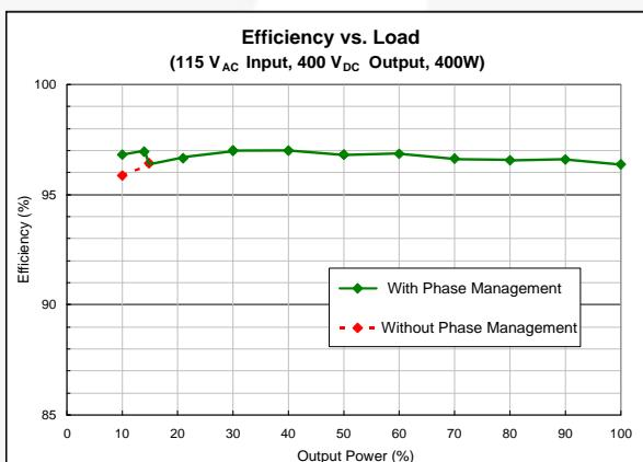
Figure 37. Measured Efficiency at 115 V<sub>AC</sub> (Default Thresholds)
