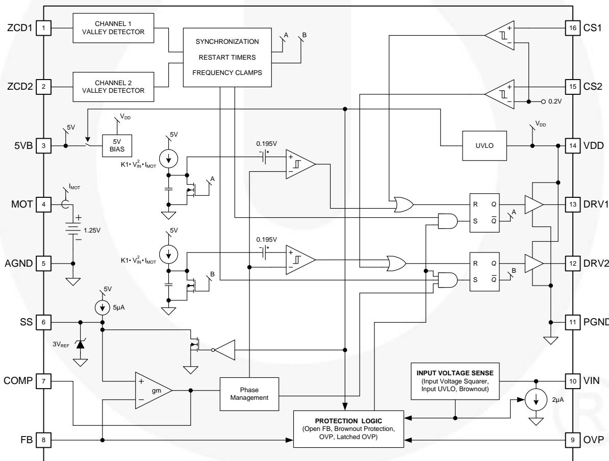
Figure 3. Block Diagram
