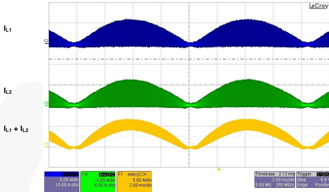
**Figure 19. Inductor Current Waveforms at Full-Load and 115 V<sub>AC</sub>**
