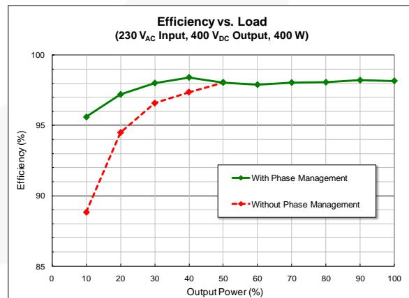
Figure 40. Measured Efficiency at 230 V<sub>AC</sub> (Adjusted Thresholds)
