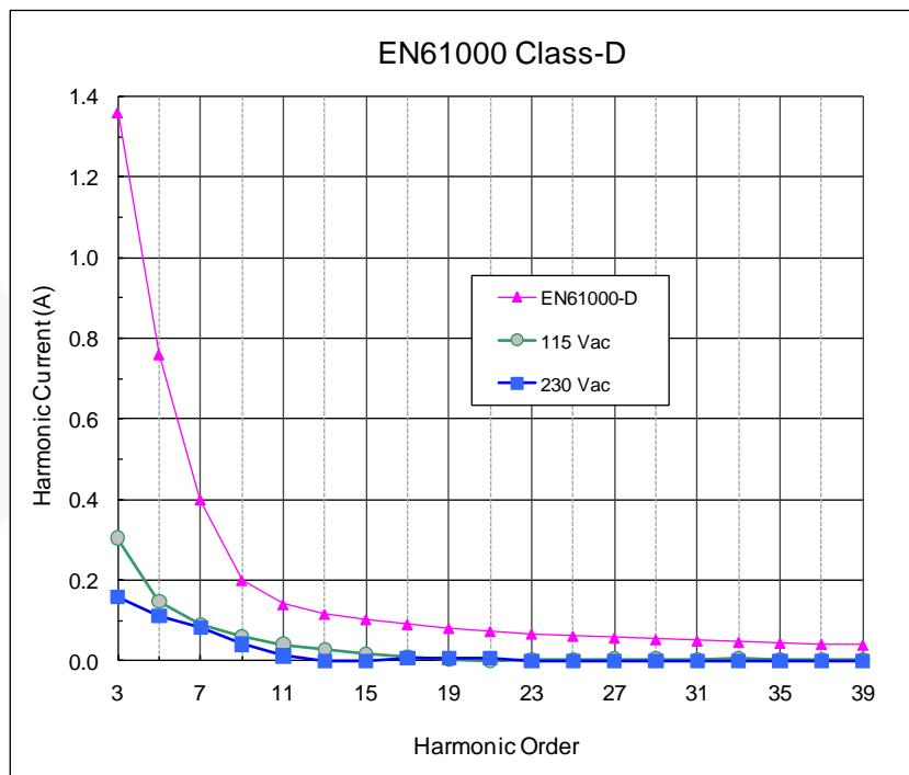
Figure 41. Measured Harmonic Current and EN61000 Class-D Regulation
