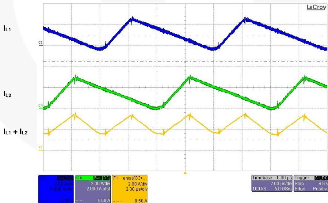
**Figure 22. Zoom of Inductor Current Waveforms of Figure 21 at Peak of Line Voltage**
