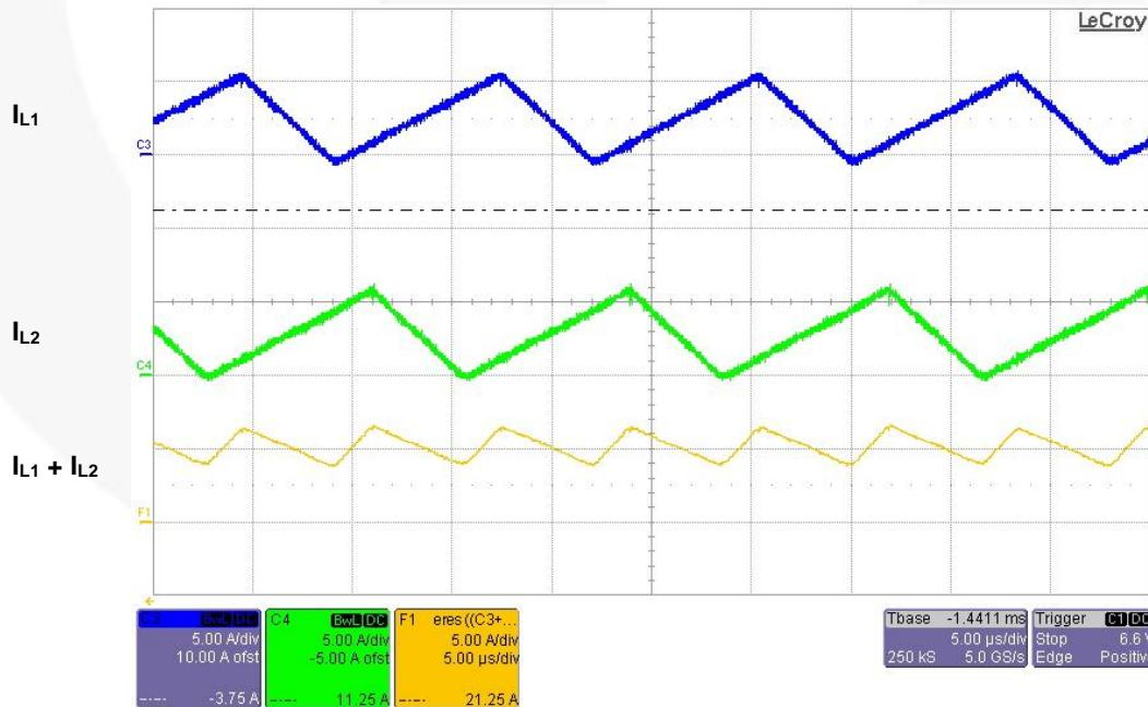
**Figure 20. Zoom of Inductor Current Waveforms of Figure 19 at Peak of Line Voltage**
