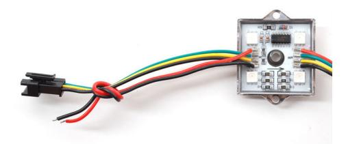
Wiring is pretty easy since there are only 4 wires. The only important thing is that you should not try to power the LED
