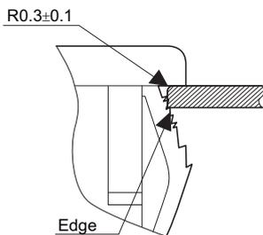
Process the above-mentioned R on the mounting hole side of panel, or be sure that the Play R is on the operation side of panel when using.
