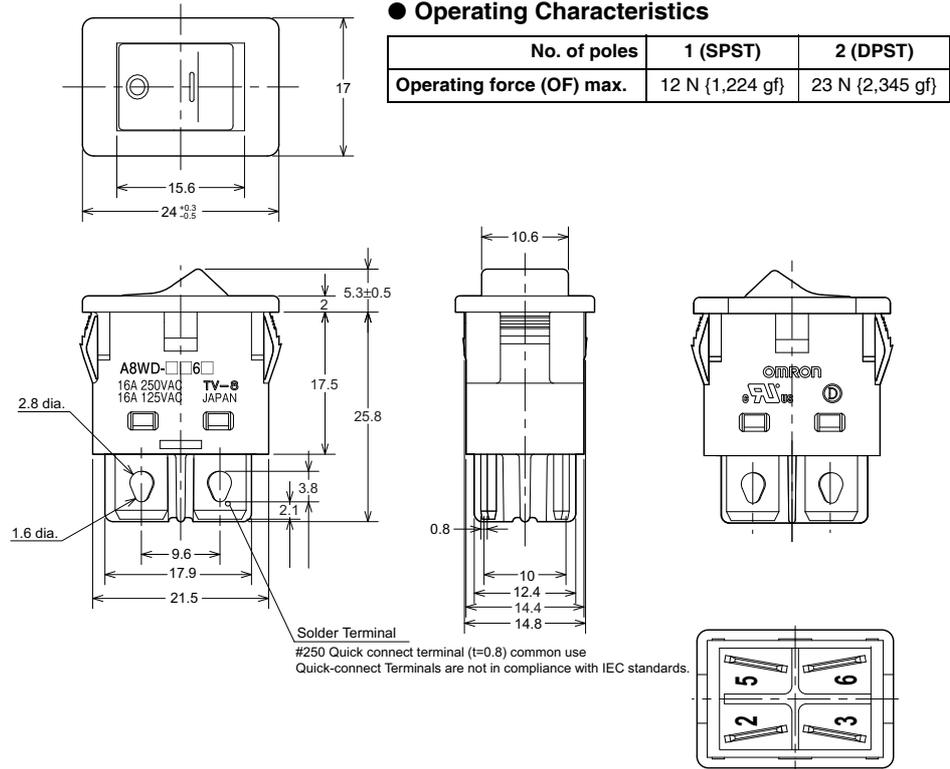
**Note:** Unless otherwise specified, a tolerance of ±0.3 mm applies to all dimensions.
