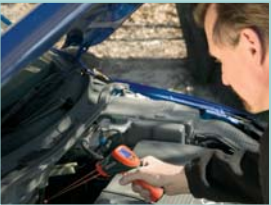
Max hold indicates and holds the peak temperature for easy identification of hot spots
