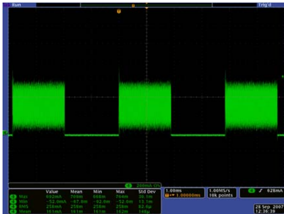
FIGURE 11. IL AT 50% PWM DIMMING
