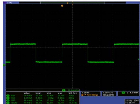
FIGURE 16. I LED AT 50% PWM DIMMING
