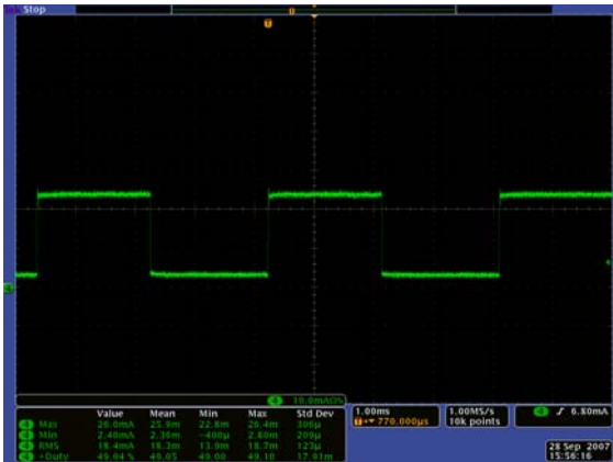
FIGURE 16. I LED AT 50% PWM DIMMING
