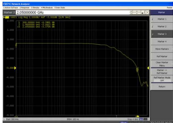
Figure 17. MHL Path SDD21 Insertion Loss Curve
