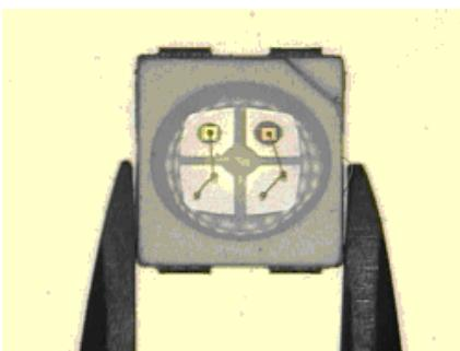
(3) When populating boards in SMT production, there are basically no restrictions regarding the form of the pick and place nozzle, except that mechanical pressure on the surface of the resin must be prevented. This is assured by choosing a pick and place nozzle which is larger than the LED's reflector area.
