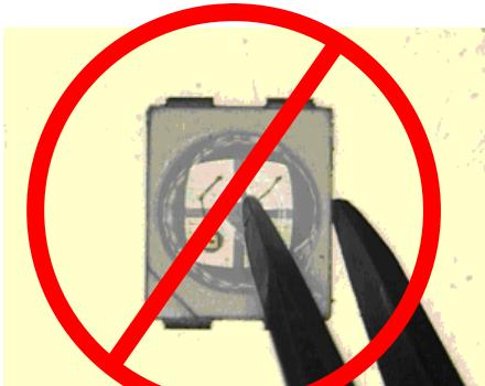
(2) In general, LEDs should only be handled from the side. By the way, this also applies to LEDs without a silicone sealant, since the surface can also become scratched.
