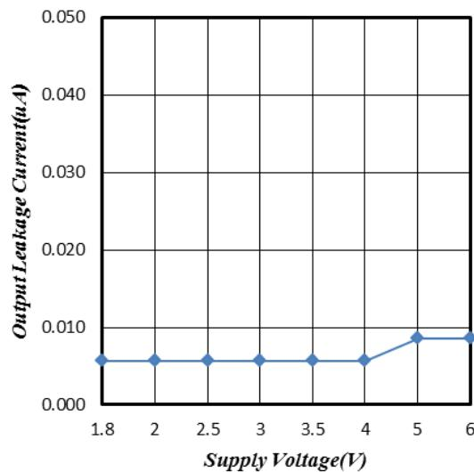
**Figure 7. Output Leakage Current vs.
