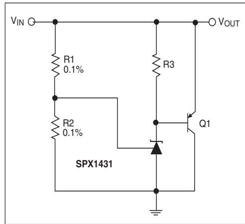
**Figure 24. High Current Shunt Regulator**
