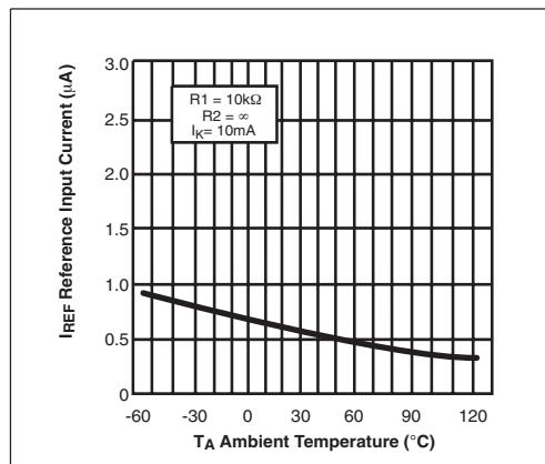
Figure 8. Reference Input Current VS Ambient Temperature
