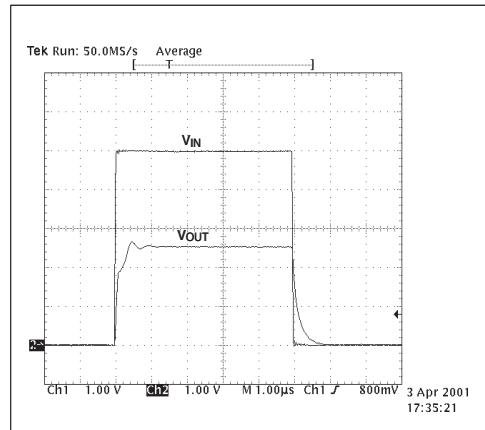
Figure 14. Frequency = 100kHz,  $I_K = 10\text{mA}$ ,  $T_A = 25^\circ\text{C}$
