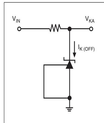
Figure 2. Test Circuit for  $V_{KA} = V_{REF}$
