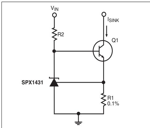
Figure 21. Constant Current, Sink,  $I_{SINK} = V_{REF}/R1$
