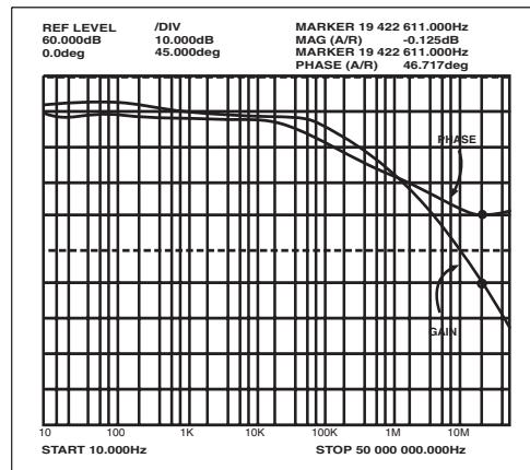
Figure 12. Small Signal Gain and Phase VS Frequency;  $I_K = 10\text{mA}$ ,  $T_A = 25^\circ\text{C}$
