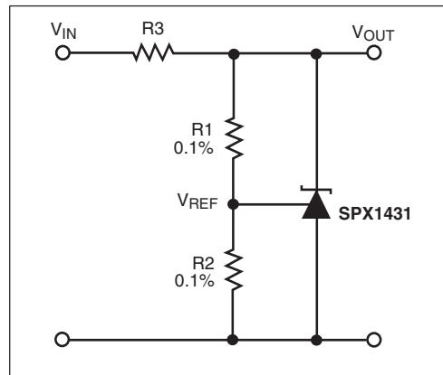
Figure 20. Shunt Regulator  $V_{OUT} = (1 + R1/R2)V_{REF}$
