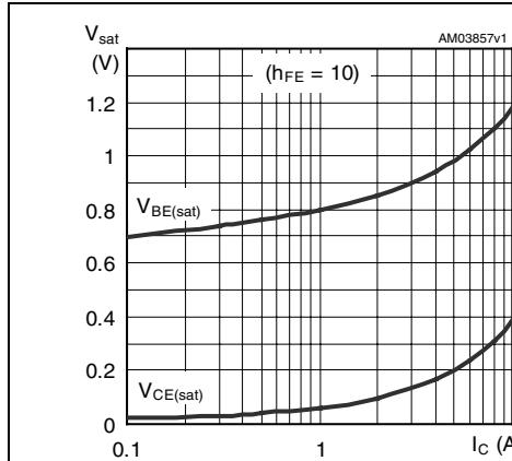
**Figure 5. Saturation voltage (PNP)**
