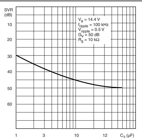
**Figure 13. Supply voltage rejection vs.  $C_2$  and  $C_3$ ,  $G_V = 390/1\Omega$**
