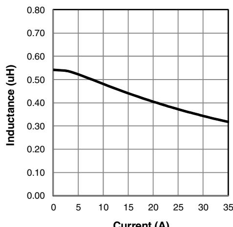
Figure 11: Inductance versus Current
