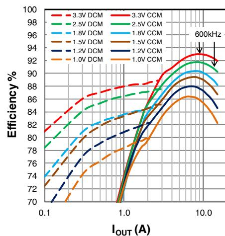
Figure 21: Efficiency,  $V_{IN}=12\text{V}$
