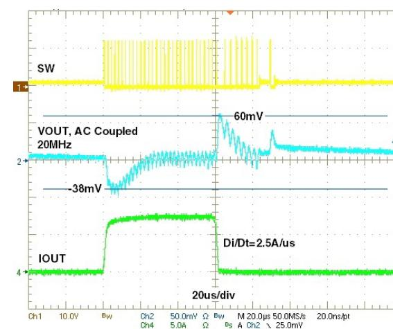
Figure 18: Load step, DCM/CCM, 0A-7.5A-0A
