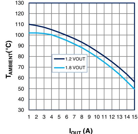
Figure 24: Maximum  $T_{AMBIENT}$  vs  $I_{OUT}$ ,  $V_{IN}=19.6\text{V}$
