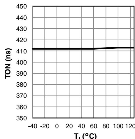
Figure 10:  $T_{ON}$  versus temperature,  $R_{ON}=16.2\text{k}\Omega$
