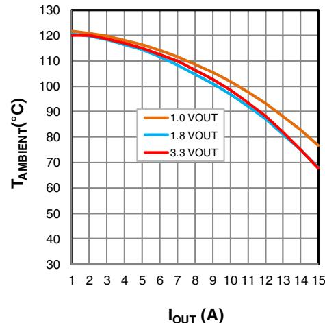
Figure 20: Maximum  $T_{AMBIENT}$  vs  $I_{OUT}$ ,  $V_{IN}=5\text{V}$
