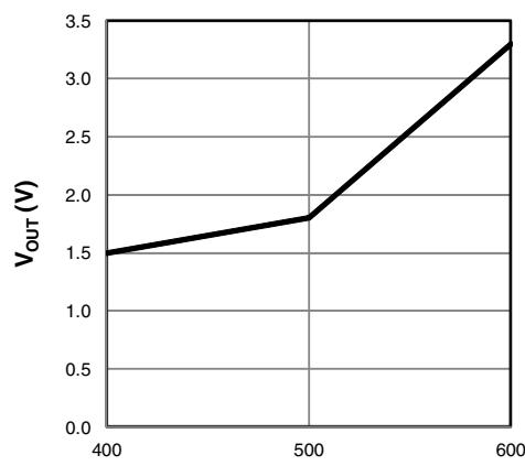
Figure 12: Maximum recommended  $V_{OUT}$  versus  $f$ ,  $V_{IN}=12V$
