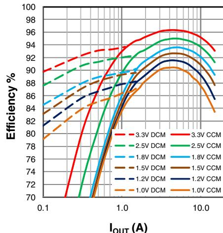
Figure 19: Efficiency,  $V_{IN}=5\text{V}$
