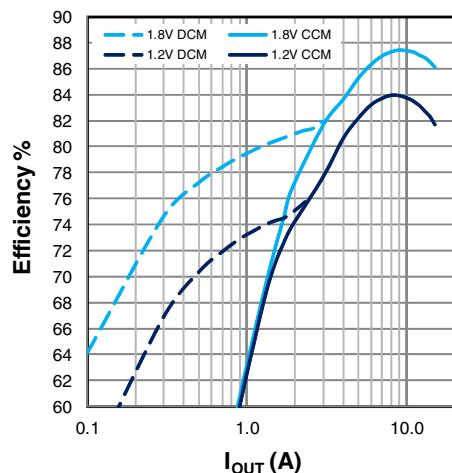
Figure 23: Efficiency,  $V_{IN}=19.6\text{V}$
