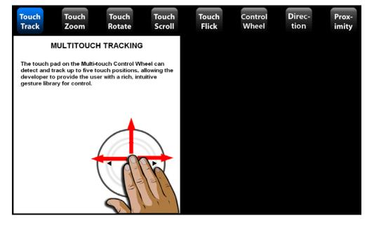
In the "Touch Track" demo function, touch the touch pad with up to five fingers and watch as your finger positions are tracked on the screen. Doubletapping on the MTCW's up/down arrows at this point alternately toggles between regular and persistent tracking mode.
