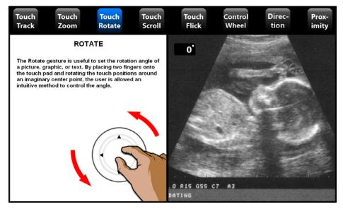
"Touch Rotate" is performed by rotating two touches about each other. It can be useful for rotating pictures, graphics or text on the screen. Note: this demo was realized using Grayhill's Instinct Gesture Recognition Library. Instinct can calculate the angle as two touch positions are rotated about each other.
