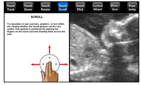
"Touch Scroll" is a two-finger gesture that allows the user to pan a picture, text or graphic. Note that the picture can be panned with momentum. To do this, try lifting your fingers as you move them across the touchpad. This is very useful when panning a large picture or searching a long list.
