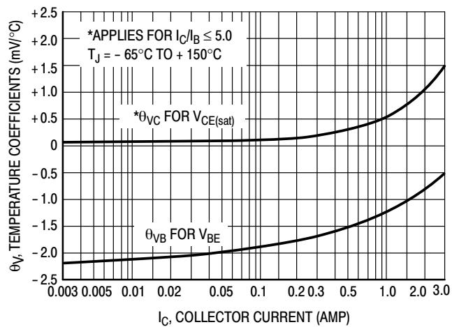
**Figure 11. Temperature Coefficients**
