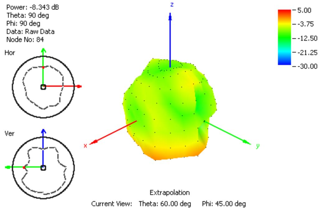
**Figure 15.** Radiation pattern at 915 MHz, Figure 1 as reference (dB), with 2m RG174 cable and 30x30 cm metal plate.
