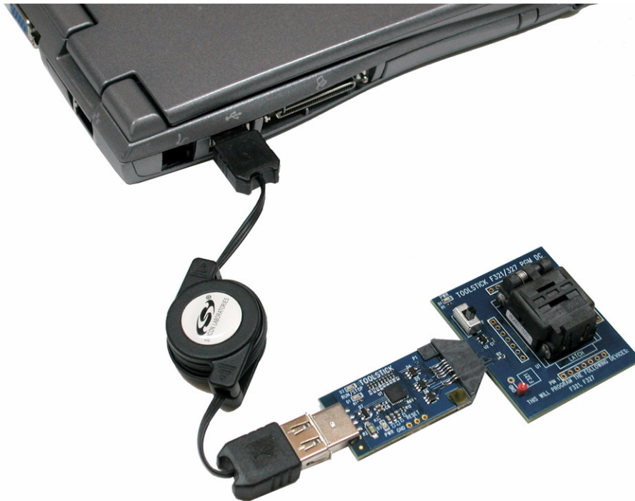
Figure 5. ToolStick Socket Platform Connected to PC
