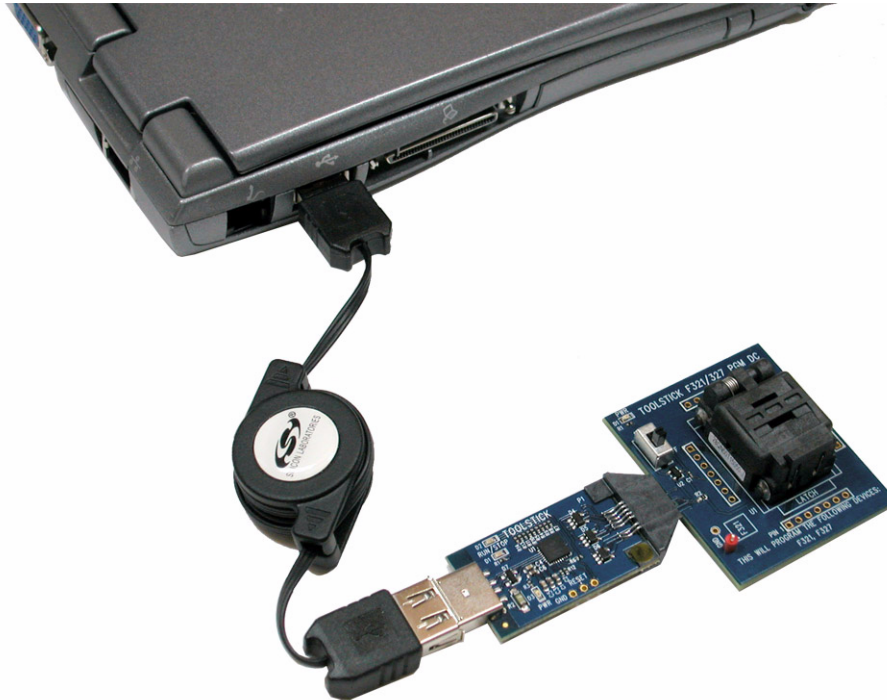
Figure 5. ToolStick Socket Platform Connected to PC
