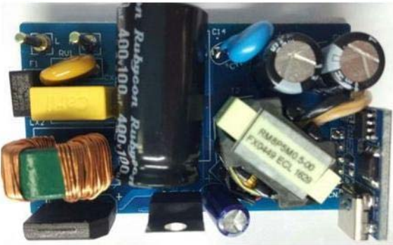
Figure 2: EVX2001-Y-02A Evaluation Board
