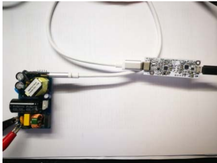
Figure 7: EVKT-MPX2001-45-PD Hardware Setup
