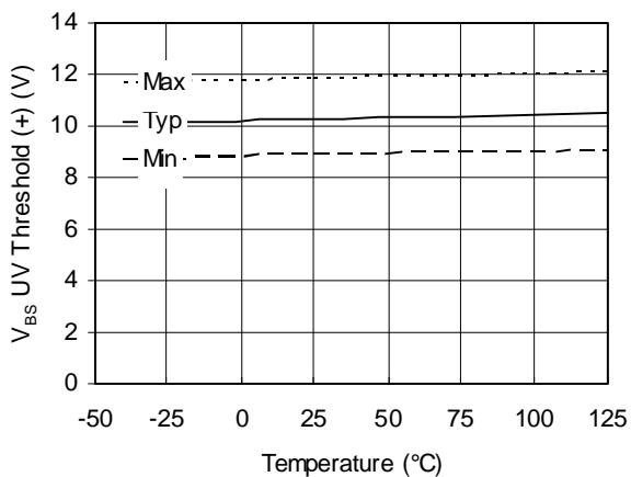
**Figure 25A. V<sub>BS</sub> UV Threshold (+) vs. Temperature**
