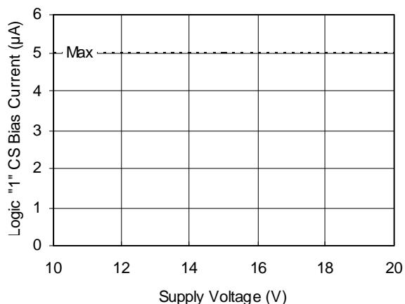
**Figure 23B. Logic "1" CS Bias Current vs. Voltage**
