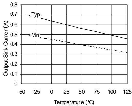
**Figure 28A. Output Sink Current vs.
