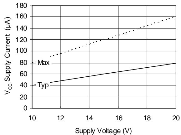
Figure 20B. V<sub>cc</sub> Supply Current vs. Voltage
