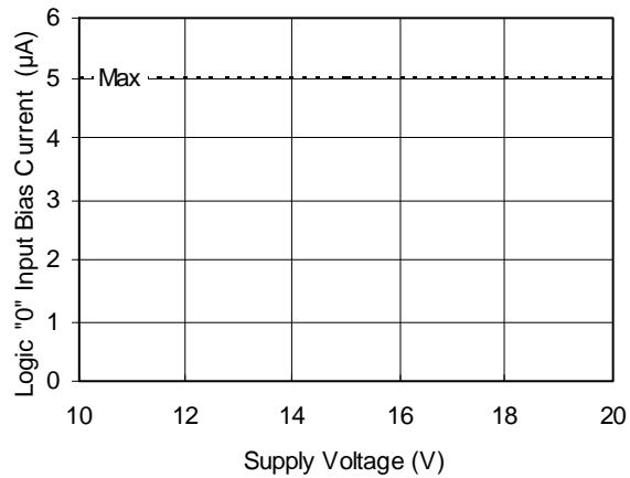
**Figure 22B. Logic "0" Input Bias Current vs. Voltage**
