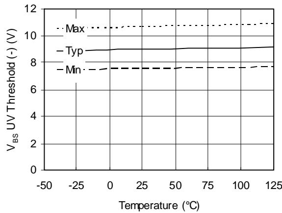
Figure 26A.  $V_{BS}$  UV Threshold (-) vs. Temperature
