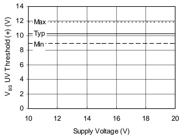
**Figure 25B. V<sub>BS</sub> UV Threshold (+) vs. Voltage**
