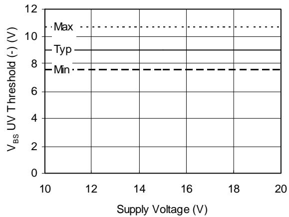
Figure 26B.  $V_{BS}$  UV Threshold (-) vs. Voltage
