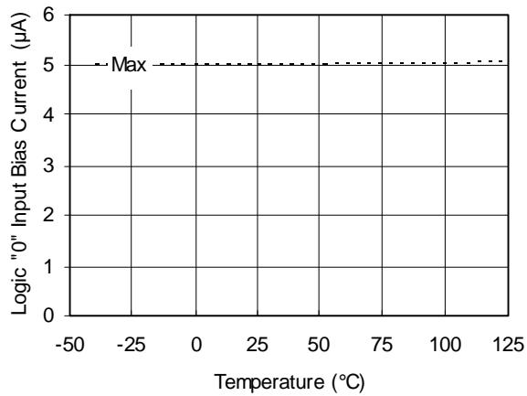
**Figure 22A. Logic "0" Input Bias Current vs. Temperature**
