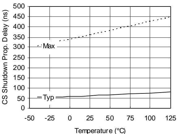
Figure 11A. CS Shutdown Prop. Delay vs. Temperature
