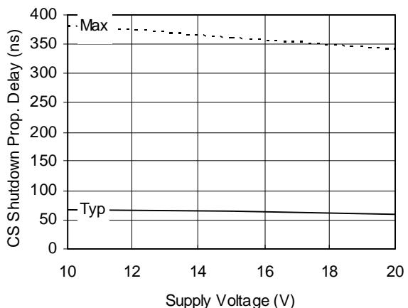
Figure 11B. CS Shutdown Prop. Delay vs. Voltage
