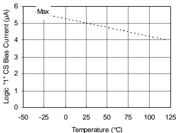
**Figure 23A. Logic "1" CS Bias Current vs. Temperature**
