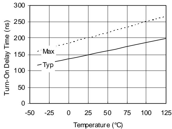
Figure 6A. Turn-On Delay Time vs.
