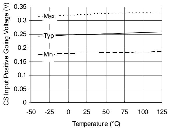
Figure 15A. CS Input Positive Going Voltage vs. Temperature
