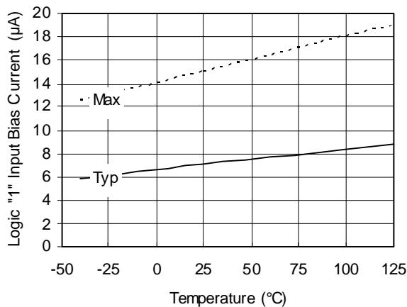
Figure 21A. Logic "1" Input Bias Current vs.
