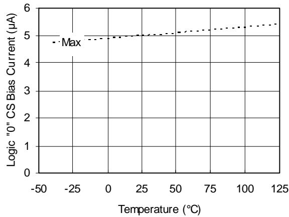
**Figure 24A. Logic "0" CS Bias Current vs. Temperature**
