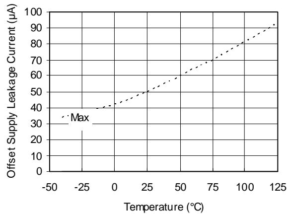
Figure 18A. Offset Supply Leakage Current vs. Temperature
