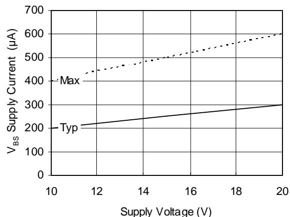
Figure 19B. V<sub>BS</sub> Supply Current vs. Voltage
