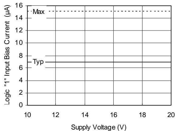
Figure 21B. Logic "1" Input Bias Current vs.
