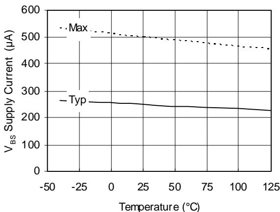
Figure 19A. V<sub>BS</sub> Supply Current vs. Temperature
