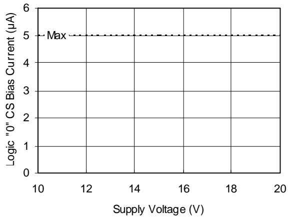
**Figure 24B. Logic "0" CS Bias Current vs. Voltage**
