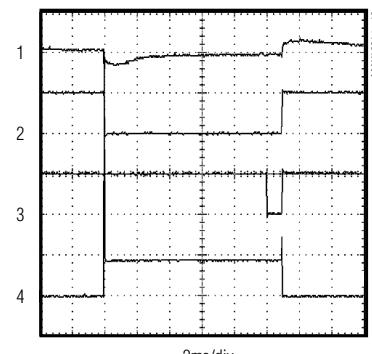
CH1 =  $V_{IN}$ , 200mV/div, AC-COUPLED; CH2 =  $V_{OUT}$ , 5V/div; CH3 =  $V_{FAULT}$ , 5V/div; CH4 =  $I_{OUT}$ , 500mA/div
