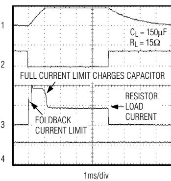
CH1 =  $V_{OUT}$ , 5V/div; CH2 =  $V_{ON}$ , 5V/div;
