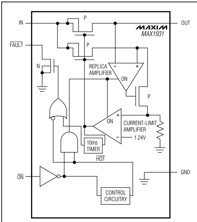
Figure 1. Functional Diagram
