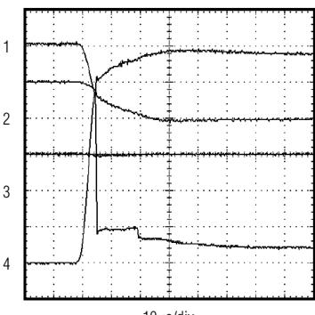
CH1 =  $V_{IN}$ , 200mV/div, AC-COUPLED; CH2 =  $V_{OUT}$ , 5V/div; CH3 =  $V_{FAULT}$ , 5V/div; CH4 =  $I_{OUT}$ , 1A/div
