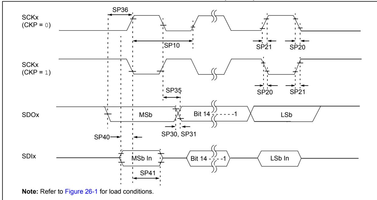
**TABLE 26-39: SPIx MASTER MODE (FULL-DUPLEX, CKE = 1, CKP = x, SMP = 1) TIMING REQUIREMENTS FOR dsPIC33FJ32(GP/MC)10X**
