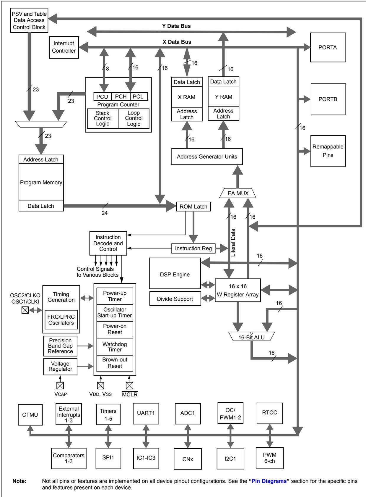
**Note:** Not all pins or features are implemented on all device pinout configurations. See the “Pin Diagrams” section for the specific pins and features present on each device.
