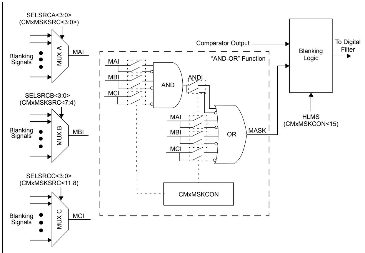
FIGURE 20-4: DIGITAL FILTER INTERCONNECT BLOCK DIAGRAM
