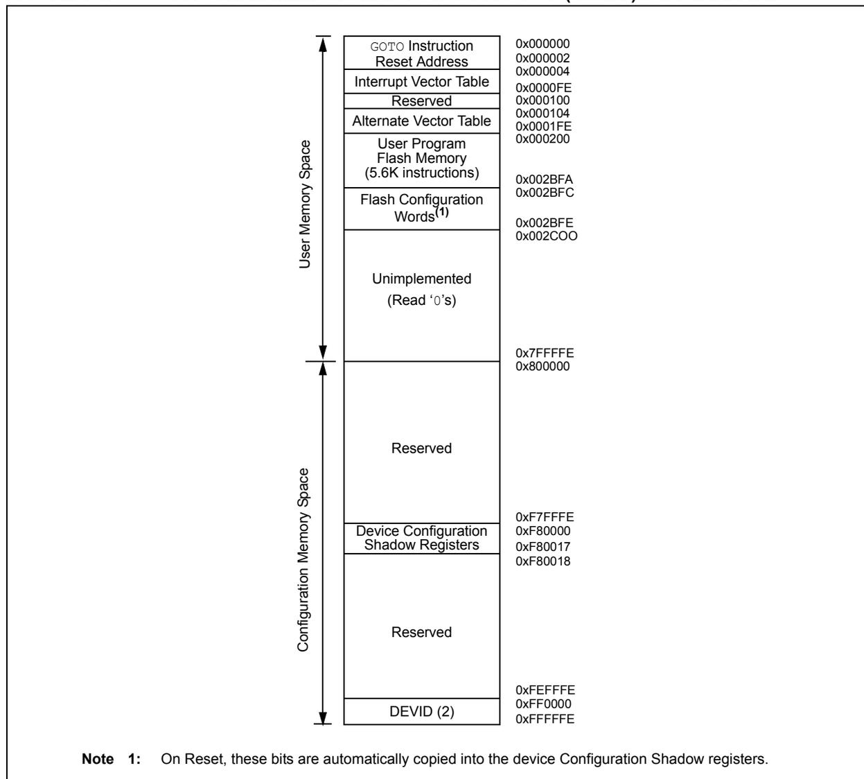
**FIGURE 4-2: PROGRAM MEMORY MAP FOR dsPIC33FJ32(GP/MC)101/102/104 DEVICES**
