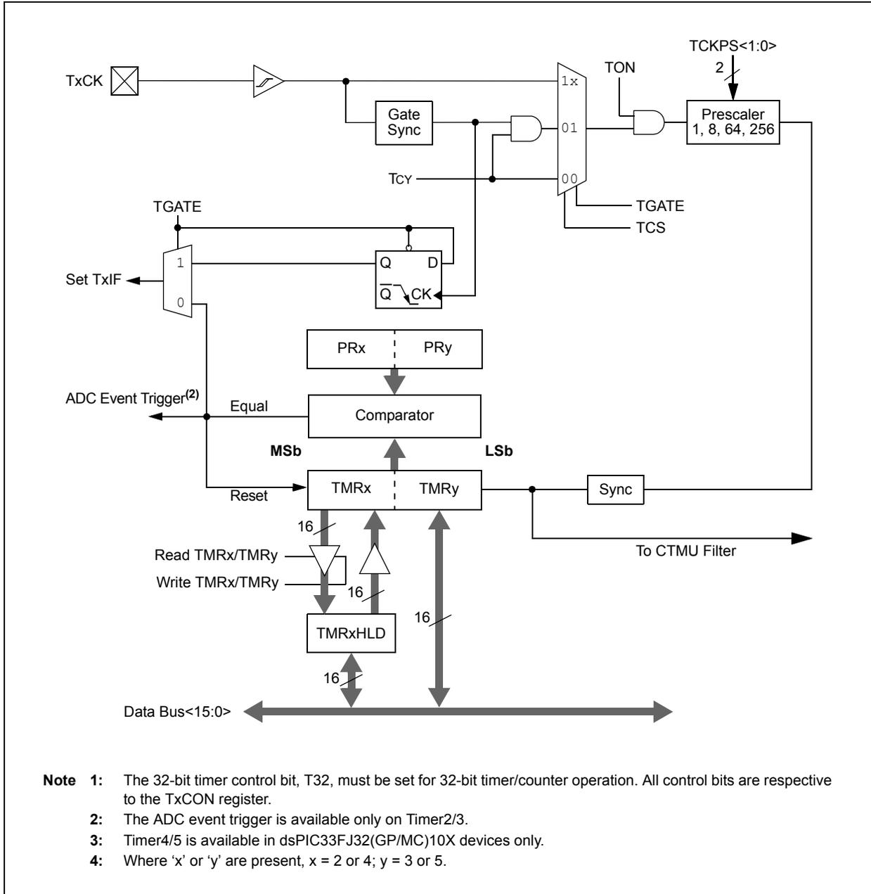
FIGURE 12-2: TIMER2 AND TIMER4 (16-BIT) BLOCK DIAGRAM<sup>(1)</sup>
