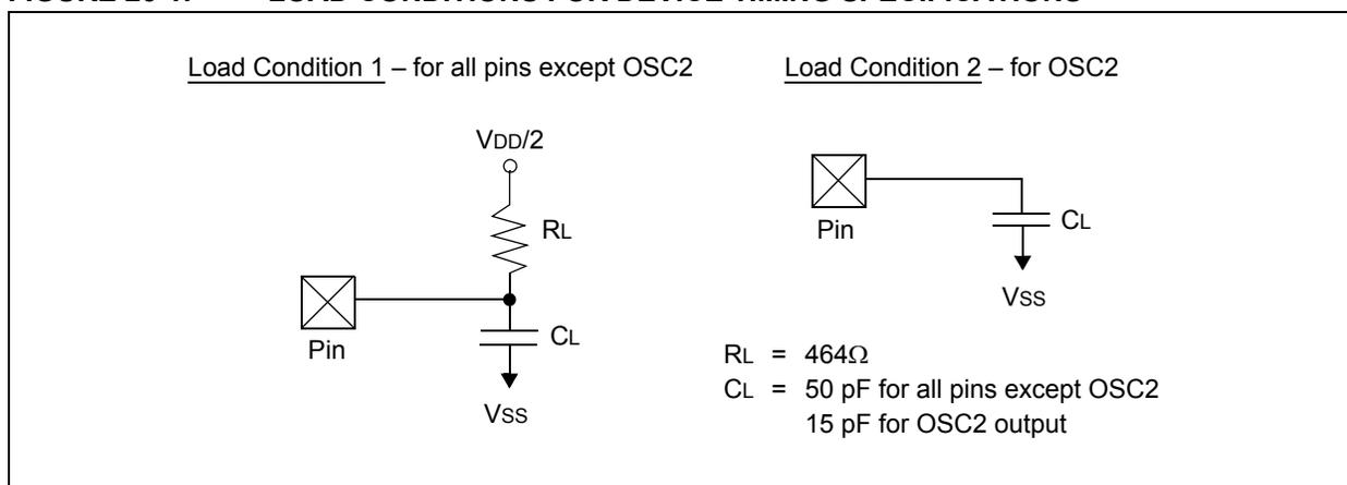
**TABLE 26-15: CAPACITIVE LOADING REQUIREMENTS ON OUTPUT PINS**
