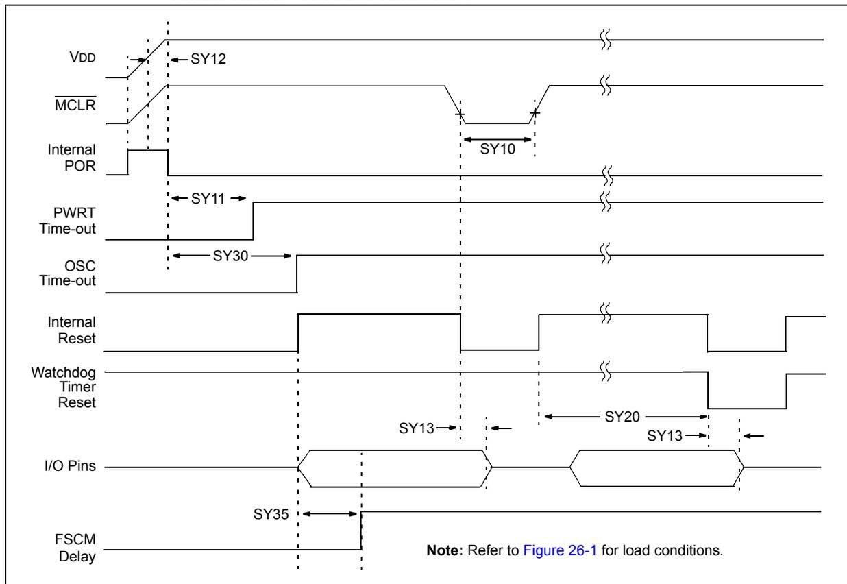
**TABLE 26-21: RESET, WATCHDOG TIMER, OSCILLATOR START-UP TIMER, POWER-UP TIMER AND BROWN-OUT RESET TIMING REQUIREMENTS**
