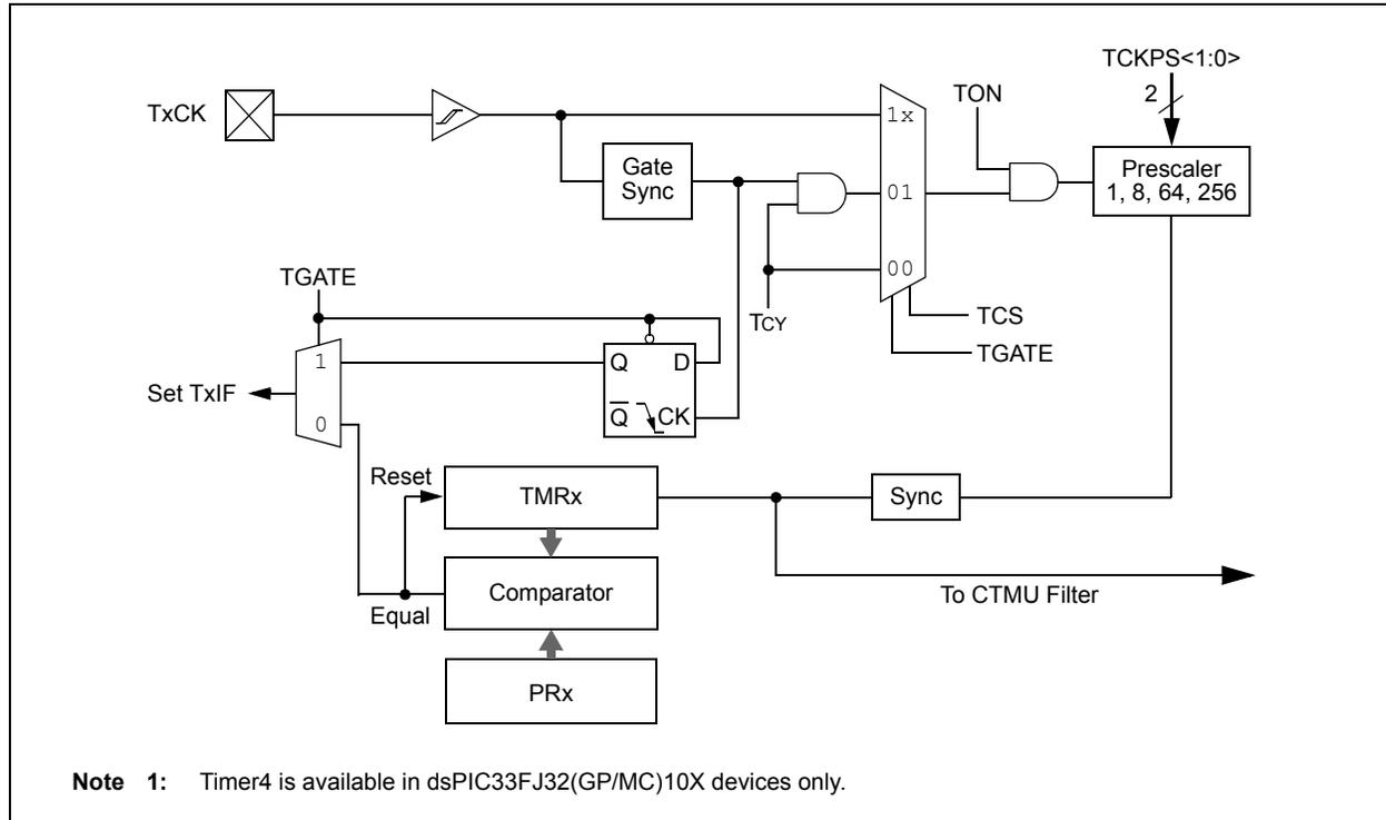
FIGURE 12-3: TIMER3 AND TIMER5 (16-BIT) BLOCK DIAGRAM<sup>(1)</sup>
