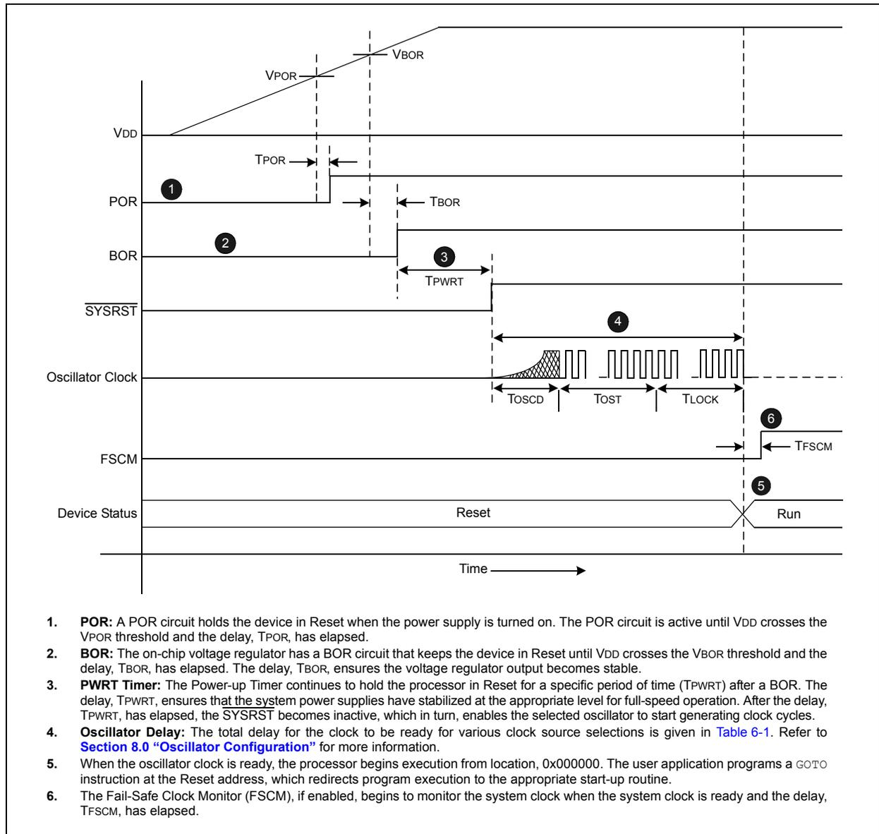
1. **POR:** A POR circuit holds the device in Reset when the power supply is turned on. The POR circuit is active until VDD crosses the VPOR threshold and the delay, TPOR, has elapsed.
