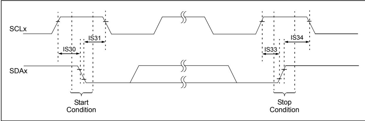
**FIGURE 26-30: I2Cx BUS DATA TIMING CHARACTERISTICS (SLAVE MODE)**
