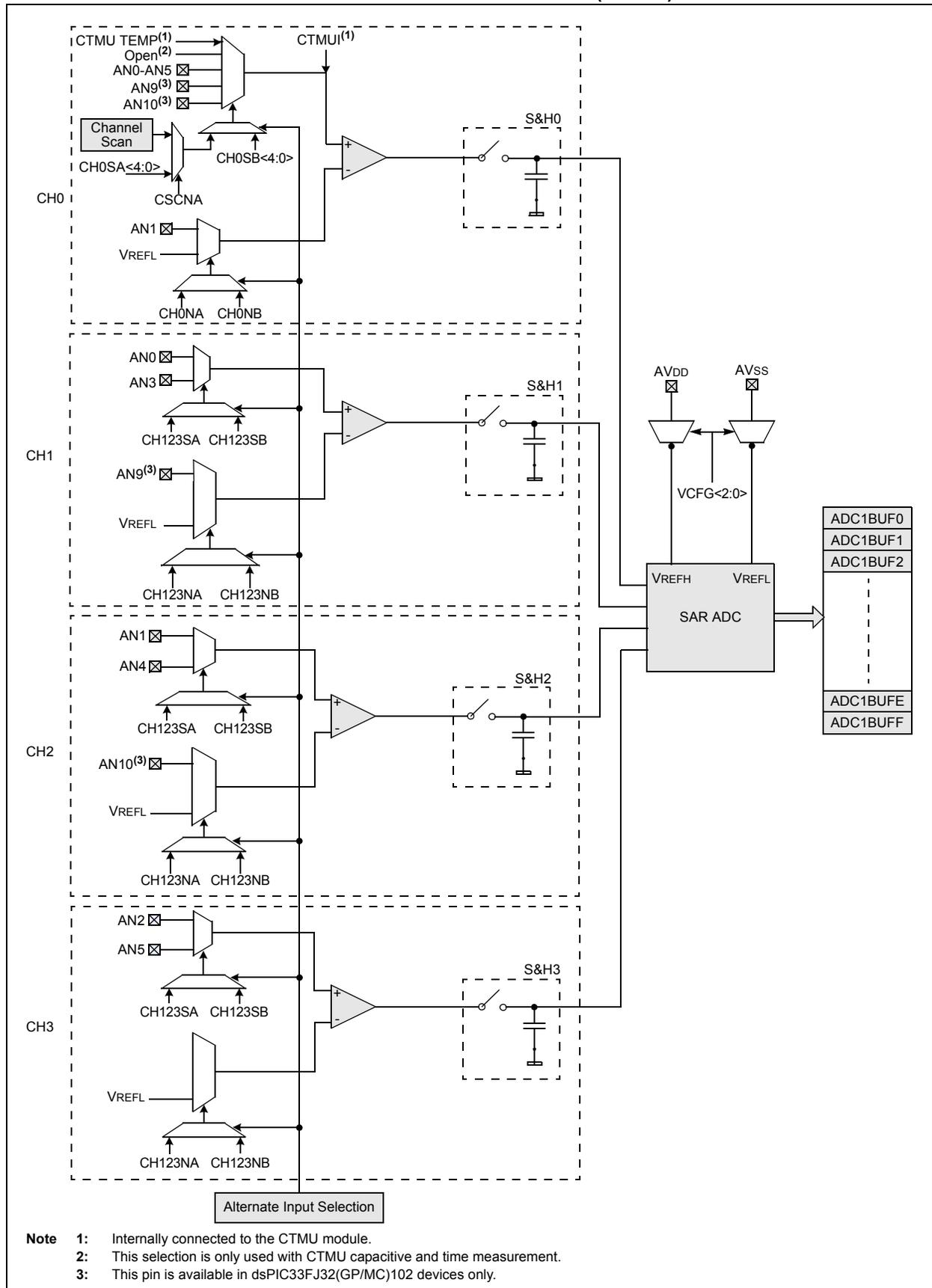
FIGURE 19-3: ADC1 BLOCK DIAGRAM FOR dsPIC33FJ32(GP/MC)104 DEVICES
