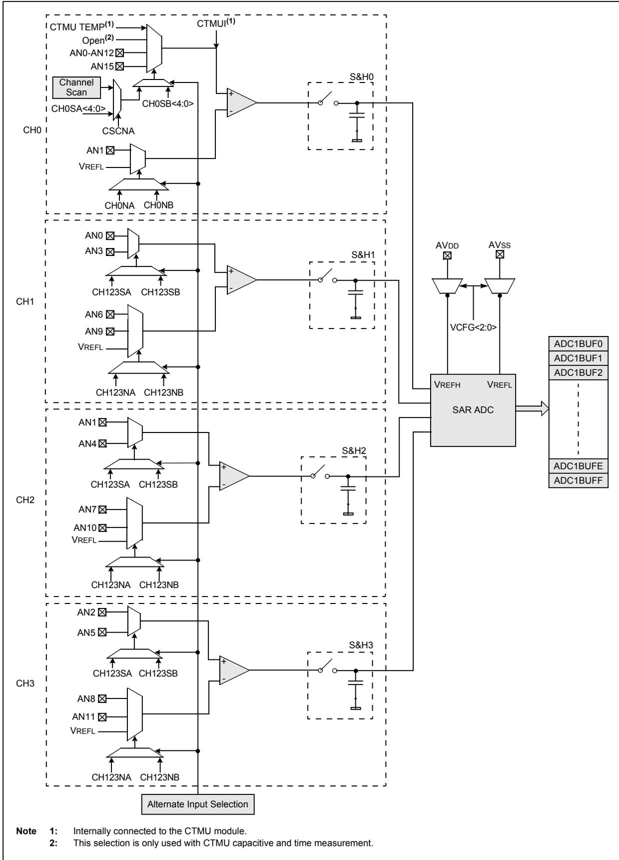
FIGURE 19-4: ADC CONVERSION CLOCK PERIOD BLOCK DIAGRAM
