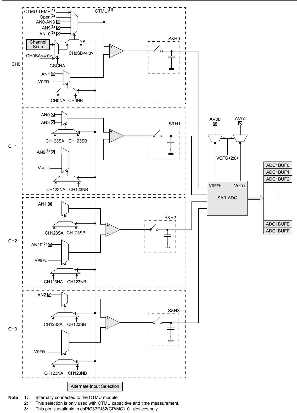
FIGURE 19-2: ADC1 BLOCK DIAGRAM FOR dsPIC33FJXX(GP/MC)102 DEVICES
