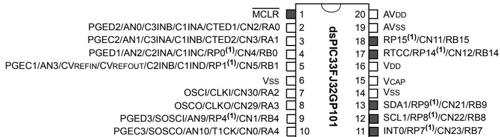
**Note 1:** The RPn pins can be used by any remappable peripheral. See [Table 1](#) for the list of available peripherals.
