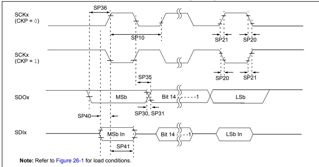
**TABLE 26-31: SPIx MASTER MODE (FULL-DUPLEX, CKE = 1, CKP = x, SMP = 1) TIMING REQUIREMENTS FOR dsPIC33FJ16(GP/MC)10X**
