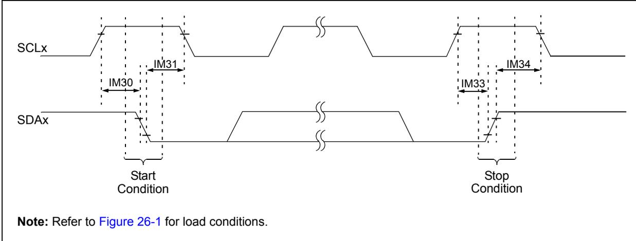
**FIGURE 26-28: I2Cx BUS DATA TIMING CHARACTERISTICS (MASTER MODE)**
