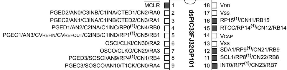
**Note 1:** The RPn pins can be used by any remappable peripheral. See [Table 1](#) for the list of available peripherals.
