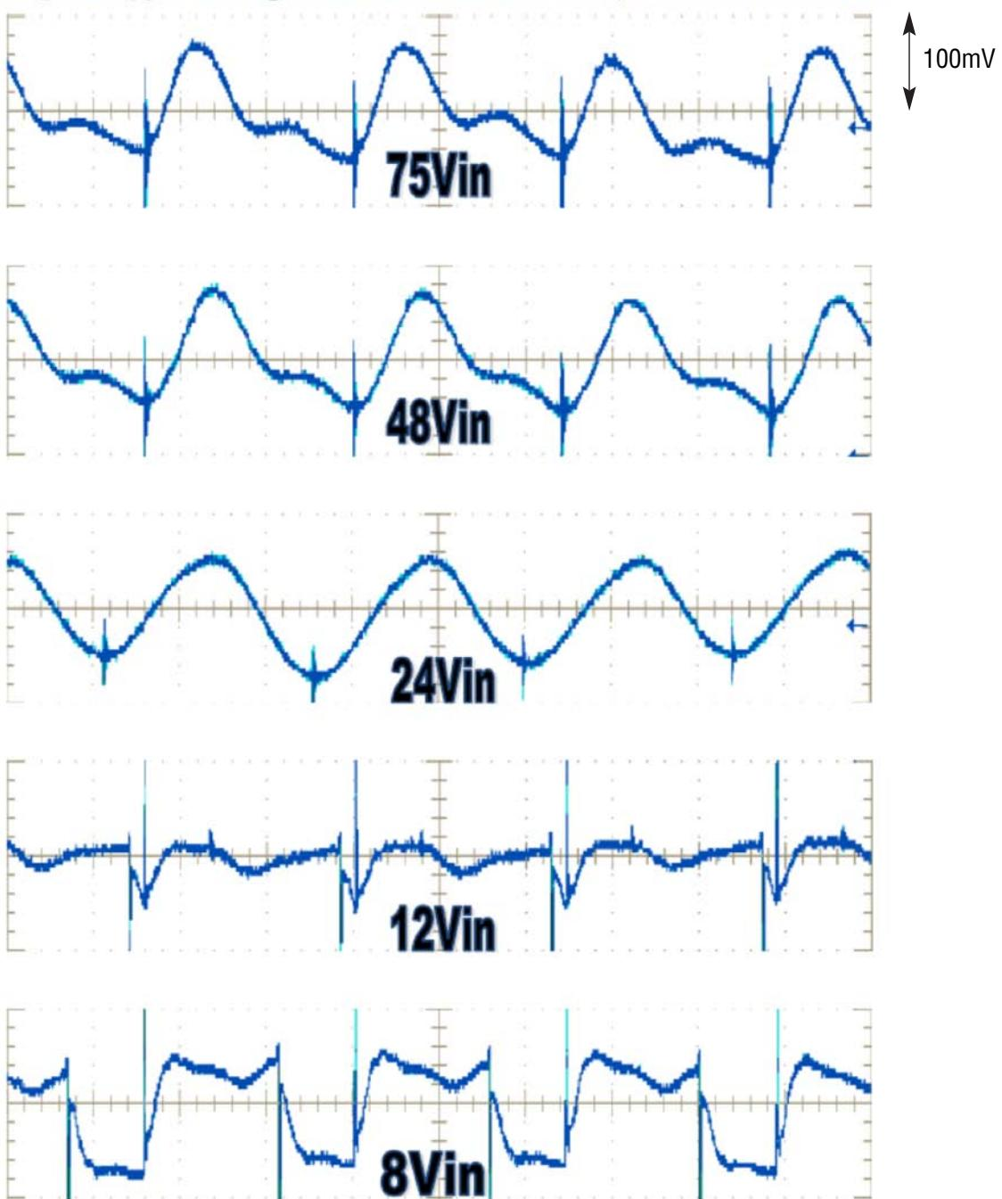
Figure 4. Output Ripple Voltage Measured Across  $C_{OUT1}$
