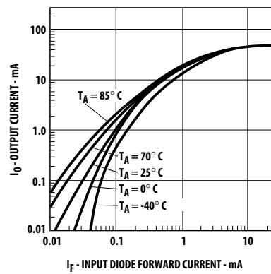
Figure 3. Output current vs. input diode forward current
