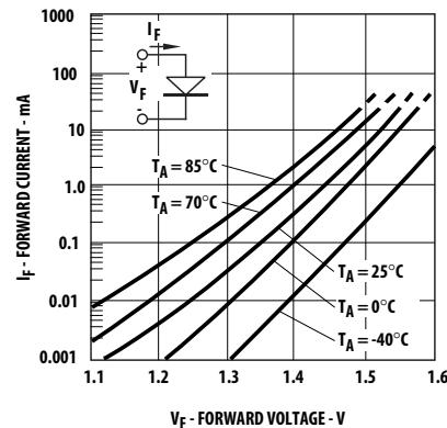
Figure 5. Input diode forward current vs. forward voltage
