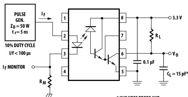
\* INCLUDES PROBE AND FIXTURE CAPACITANCE
