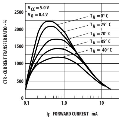
Figure 2. Current transfer ratio vs. forward current
