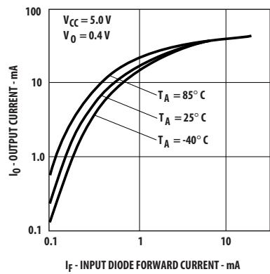
Figure 4. Output current vs. input diode forward current
