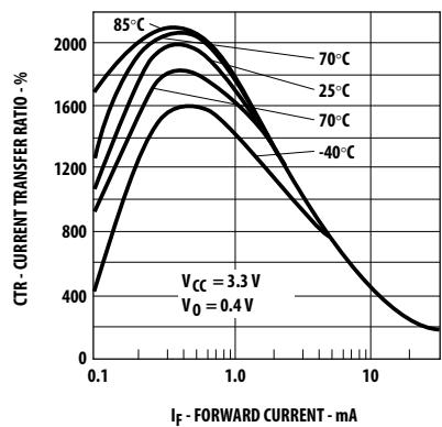
Figure 1. Current transfer ratio vs. forward current
