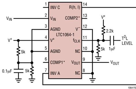
Figure 3. Level Shifting the Input T<sup>2</sup>L Clock for Single Supply Operation, V<sub>+</sub> > 6V.
