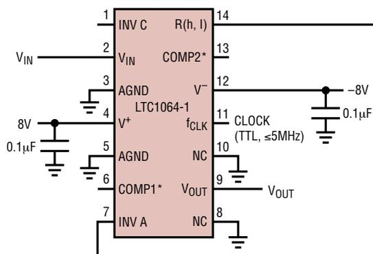
NOTE: THE POWER SUPPLIES SHOULD BE BYPASSED BY A  $0.1\mu\text{F}$  CAPACITOR CLOSE TO THE PACKAGE.
