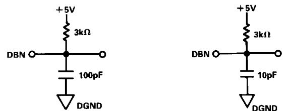
a. High-Z to V OL b. V OL to High-Z Figure 5. Load Circuit for \overline{INT} Propagation Delays
