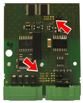
Figure 49: Connection of jumpers
