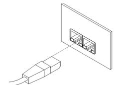
Figure 35: Connection of Ethernet cable
