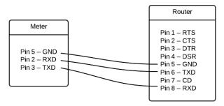
Figure 45: Meter connection to router
