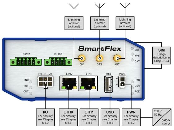
Figure 55: Router connection
