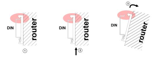
Figure 27: Removal of the DIN rail
