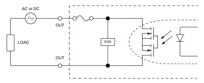
Figure 41: Binary output connection
