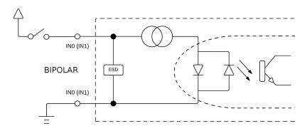
Figure 40: Binary inputs connection
