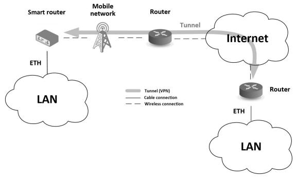
Figure 3: Using VPN tunnel
