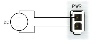
Figure 30: Connection of power supply
