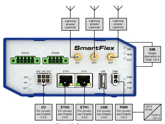
Figure 55: Router connection
