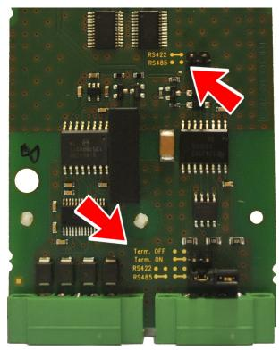
Figure 49: Connection of jumpers
