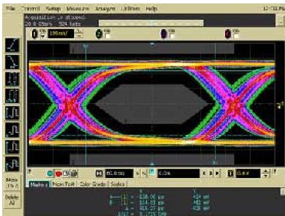
Figure 8: 12bit deep color DVI/HDMI TX eye tested with 20 meter. 24 AWG HDMI cable. Setting: Optimized equalization, 0dB output pre-emphasis and de-emphasis, and Swing 500mV.
