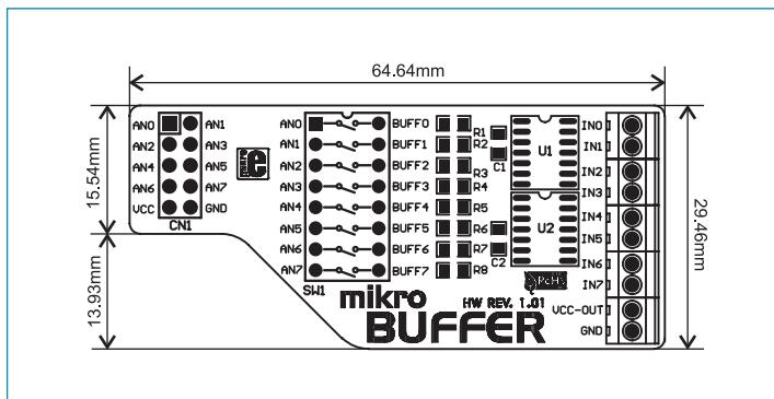
Figure 2: Dimensions of the mikroBuffer additional board
