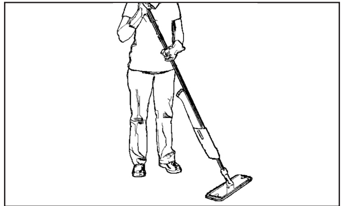
Figure 6. Applying floor finish with Flat Mop (optional)
