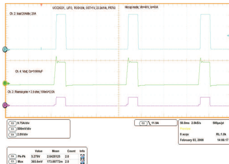
Figure 42. Cycle-by-Cycle Current Limit
