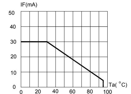
FIG.5 MAXIMUM FORWARD DC CURRENT
