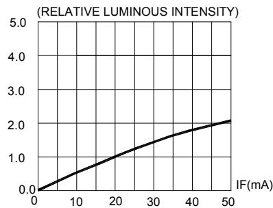
FIG.2 RELATIVE LUMINOUS INTENSITY VS.
