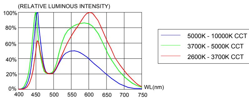
FIG.4 RELATIVE LUMINOUS INTENSITY VS.
