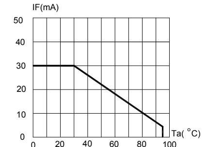
FIG.5 MAXIMUM FORWARD DC CURRENT
