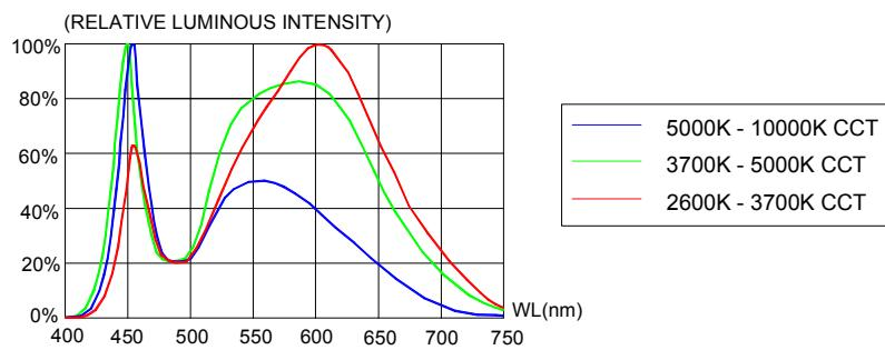
FIG.4 RELATIVE LUMINOUS INTENSITY VS.
