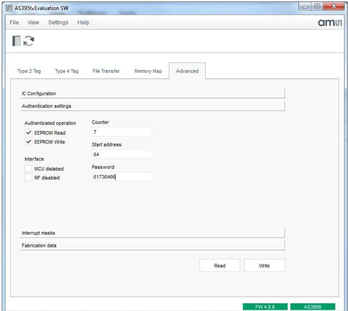
Figure 15: AS395x GUI – Advanced tab, Authentication Settings
