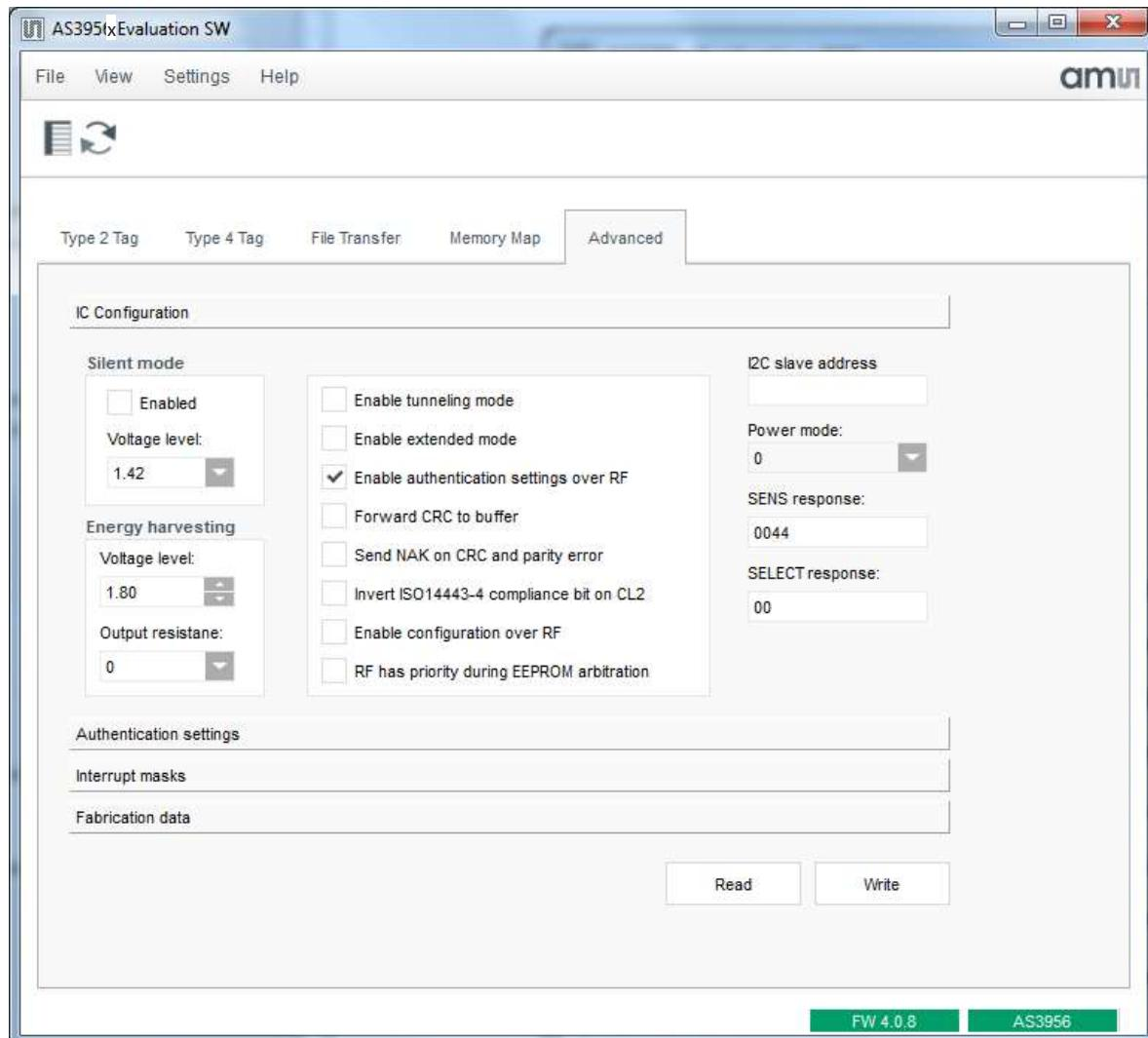
Figure 35: AS395x GUI – Enable auth settings from RF
