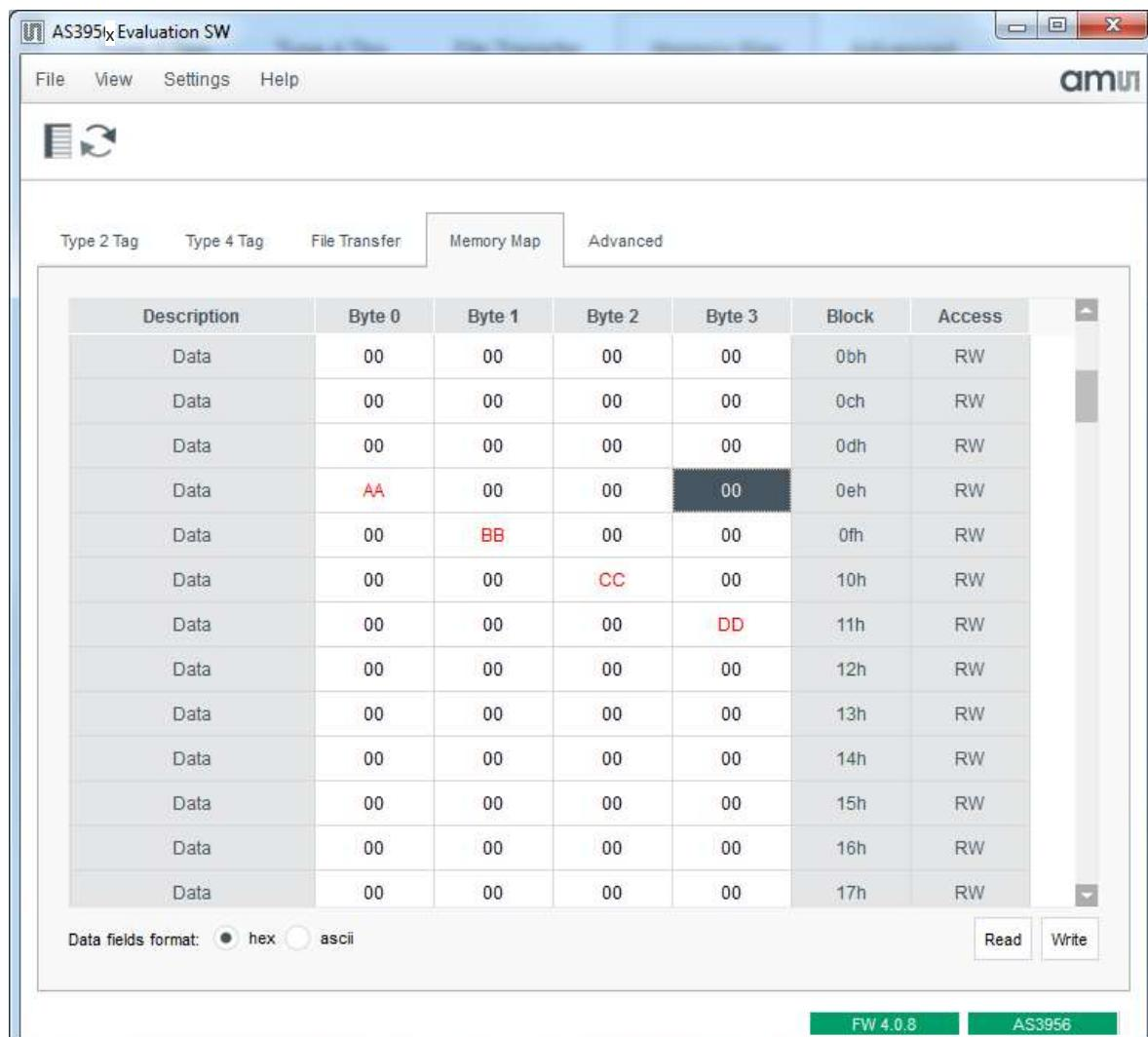
Figure 13: AS395x GUI – Memory Map tab, data enter
