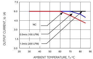
Figure 21. Derating Output Current versus Local Ambient Temperature and Airflow (Vin = 3.3Vdc, Vo=2.5 Vdc).
