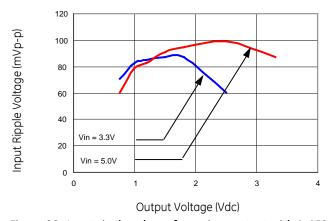
Figure 26. Input ripple voltage for various output with 1x150  $\mu$ F polymer and 1x47  $\mu$ F ceramic capacitors at the input (80% of Io,max).
