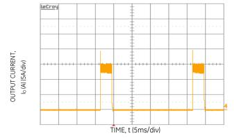
Figure 15. Typical Start-Up Using Remote On/Off with Low-ESR external capacitors (7x150uF Polymer) (Vin = 5.0Vdc, Vo = 3.3Vdc, Io = 6A, Co =  $1050\mu F$ ).
