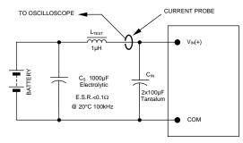
NOTE: Measure input reflected ripple current with a simulated source inductance ( $L_{TEST}$ ) of 1 $\mu$ H. Capacitor C<sub>S</sub> offsets possible battery impedance. Measure current as shown above.
