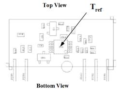
Figure 32. Tref Temperature measurement location.
