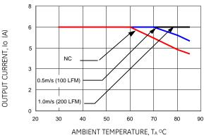
Figure 22. Derating Output Current versus Local Ambient Temperature and Airflow (Vin = 3.3dc, Vo=0.75 Vdc).
