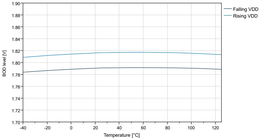
**Figure 5-40. BOD Threshold vs. Temperature (Level 2.6V)**
