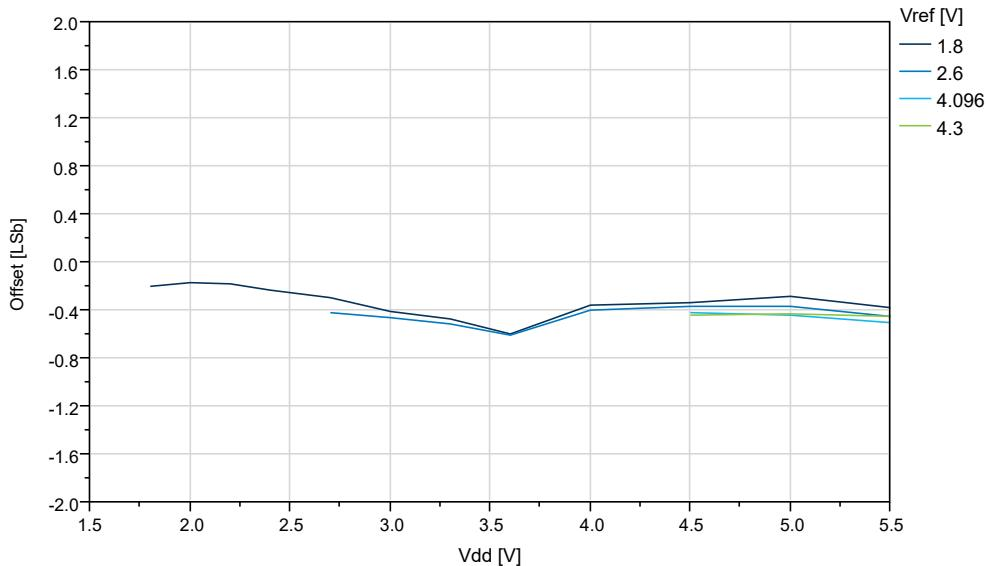
**Figure 5-61. Offset vs.  $V_{REF}$  ( $V_{DD}=5.0V$ ,  $f_{ADC}=115\text{ kspS}$ , REFSEL = External Reference)**
