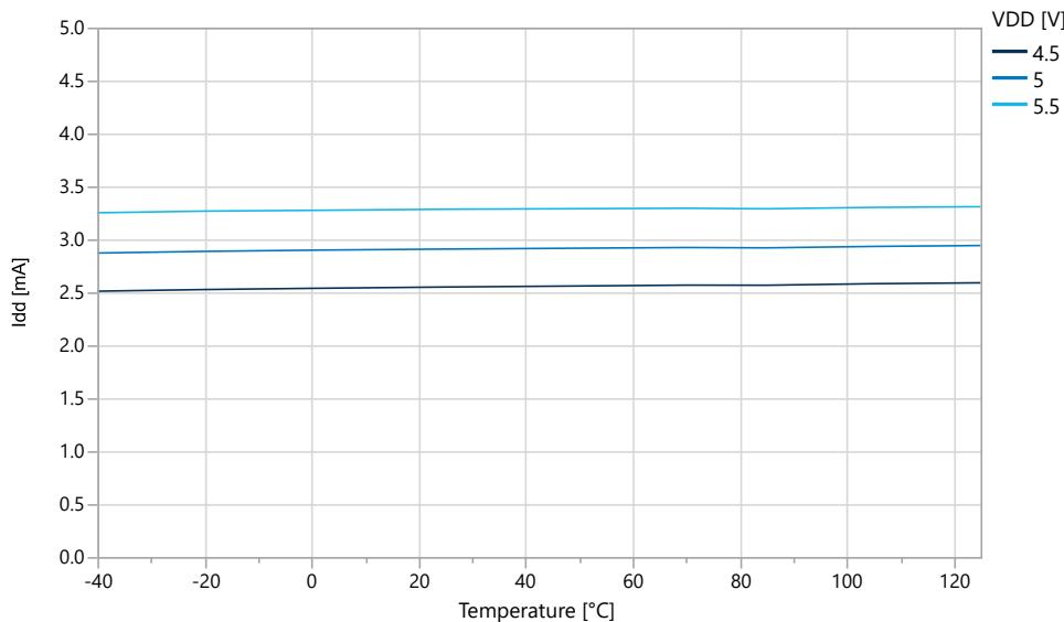
**Figure 5-9. Idle Supply Current vs.  $V_{DD}$  ( $f=32.768$  kHz OSCULP32K)**
