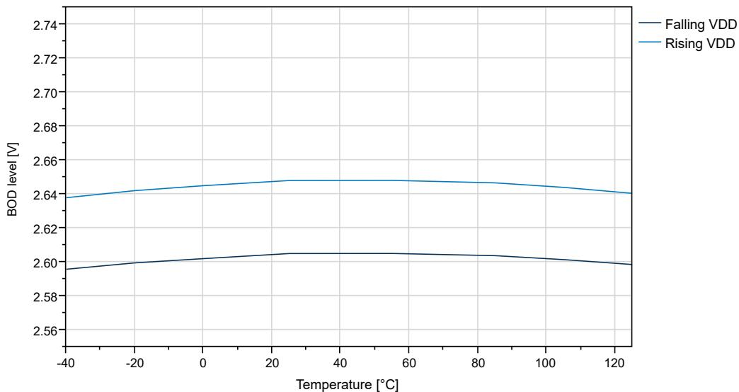
**Figure 5-41. BOD Threshold vs. Temperature (Level 4.3V)**
