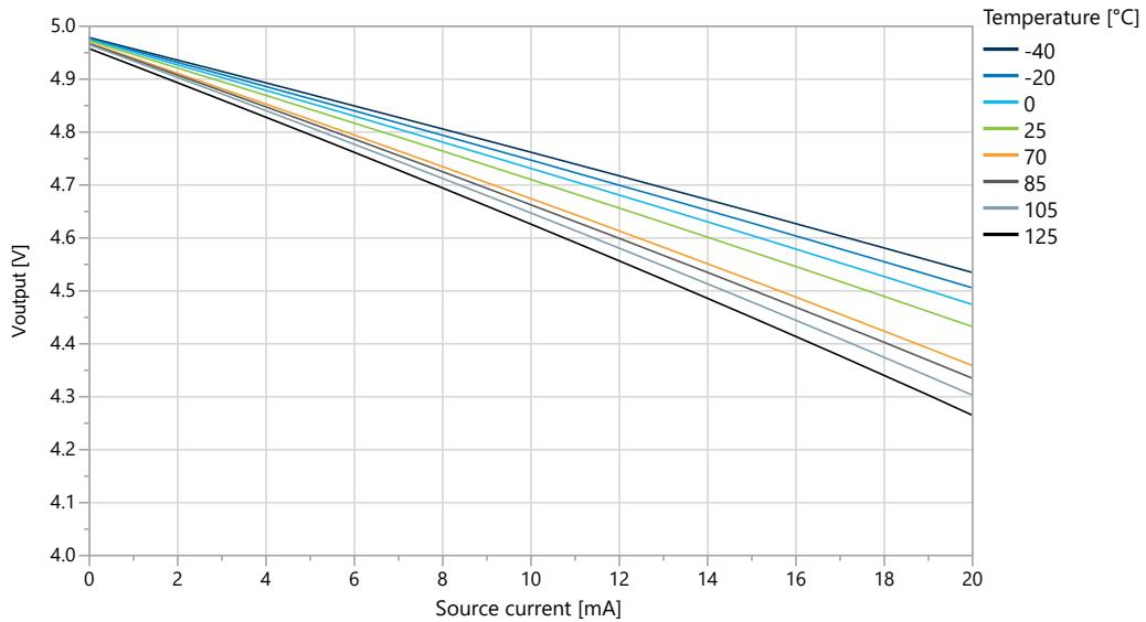
Figure 5-28. I/O Pin Output Voltage vs. Source Current (T=25°C)
