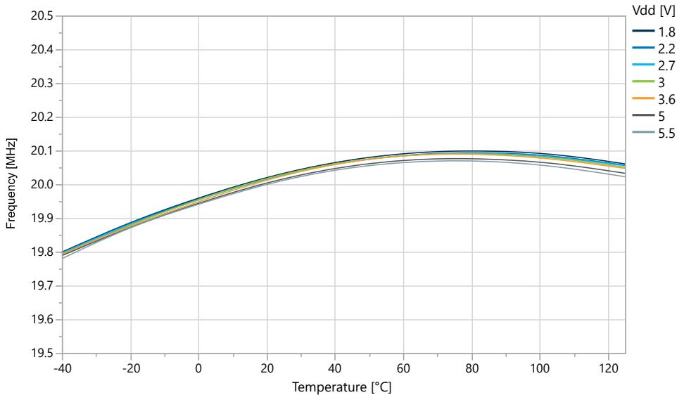
**Figure 5-69. OSC20M Internal Oscillator: Frequency vs. V<sub>DD</sub>**
