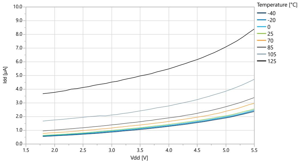
**Figure 5-14.** Standby Mode Supply Current vs. V<sub>DD</sub> (Sampled BOD running at 125 Hz)
