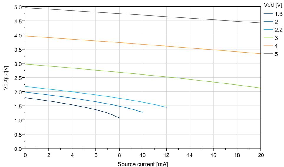
**GPIO Pull-Up Characteristics**
