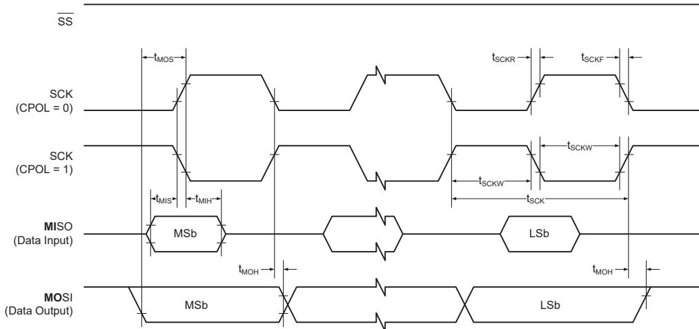
**Figure 4-5. SPI - Timing Requirements in Slave Mode**
