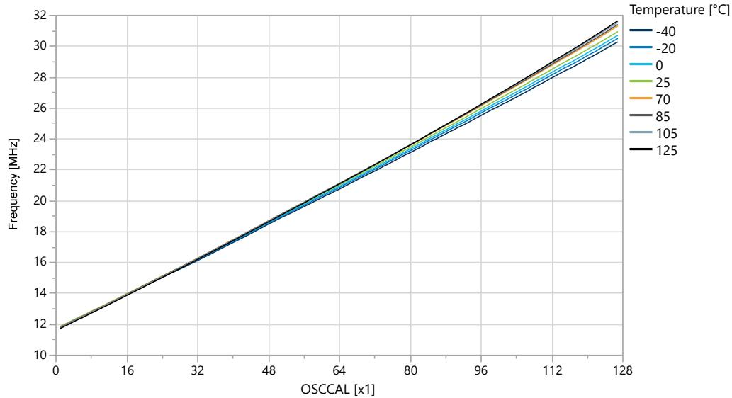
Figure 5-68. OSC20M Internal Oscillator: Frequency vs. Temperature
