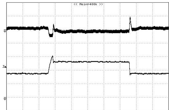
Figure 9: Output voltage response to step-change in load current (75%-50%-75% of I_{o, max} ; di/dt = 1.0A/\mu s ). Load cap: 470 \mu F POS capacitor and 1 \mu F ceramic capacitor. Top Trace: V_{out} (100mV/div, 200us/div), Bottom Trace: I_{out} (10A/div). Scope measurement should be made using a BNC cable (length shorter than 20 inches). Position the load between 51 mm to 76 mm (2 inches to 3 inches) from the module
