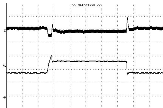
Figure 9: Output voltage response to step-change in load current (75%-50%-75% of I_o , max; di/dt = 1.0A/\mu s ). Load cap: 470 \mu F POS capacitor and 1 \mu F ceramic capacitor. Top Trace: V_{out} (100mV/div, 200us/div), Bottom Trace: I_{out} (10A/div). Scope measurement should be made using a BNC cable (length shorter than 20 inches). Position the load between 51 mm to 76 mm (2 inches to 3 inches) from the module
