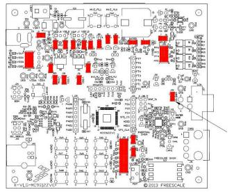
Figure 2. Jumper configuration diagram
