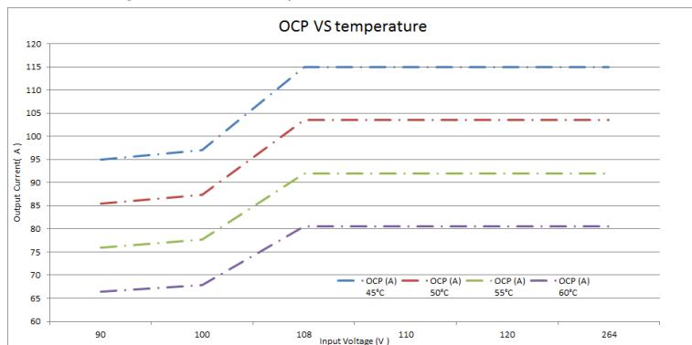
Figure 6 - Vin vs Output Current for PET1300-12-054RA
