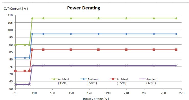
Figure 3 - Derating on  $I_{out}$  vs  $V_{in}$  and  $T_a$  for PET1300-12-054RA
