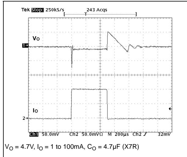
**Figure 21. Line transient response**
