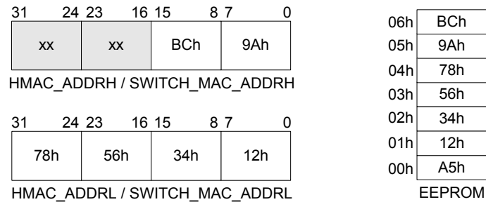
Figure 9.2 Example EEPROM MAC Address Setup
