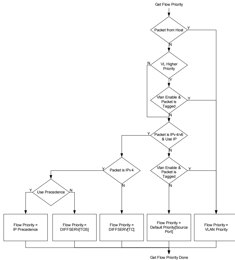
Figure 6.8 Switch Engine Ingress Flow Priority Calculation
