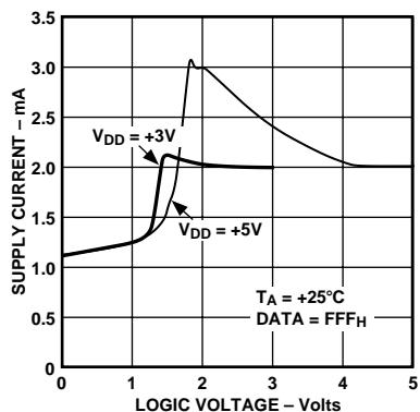
Figure 10. Supply Current vs. Logic Input Voltage
