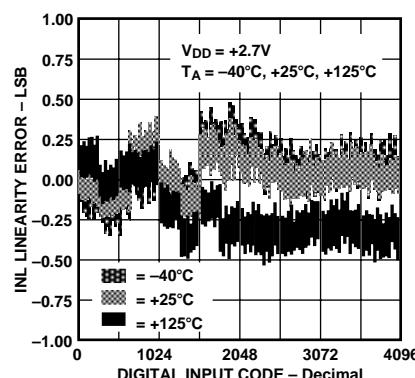
Figure 2. Linearity Error vs. Digital Code and Temperature
