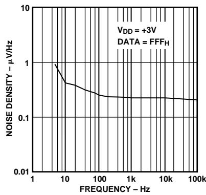
Figure 17. Output Voltage Noise Density vs. Frequency
