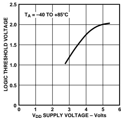
Figure 5. Logic Input Threshold Voltage vs.  $V_{DD}$
