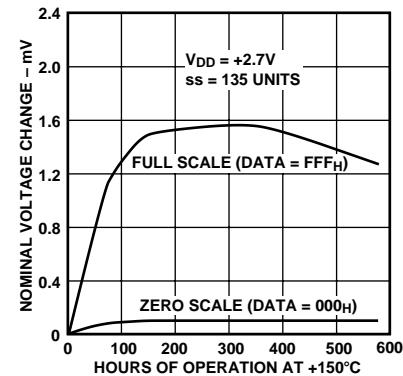
Figure 19. Long Term Drift Accelerated by Burn-In
