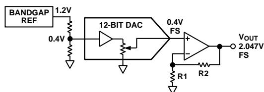
Figure 20. Equivalent AD8300 Schematic of Analog Portion
