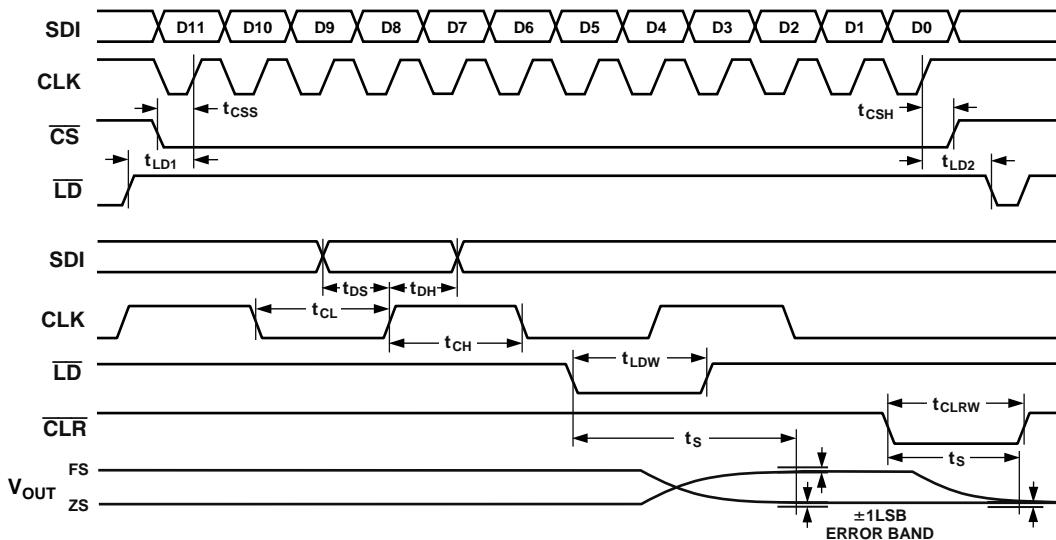
Figure 3. Timing Diagram
