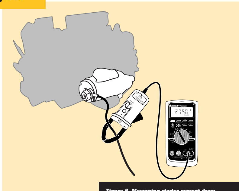
Figure 6. Measuring starter current draw
